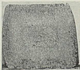
Fig. 14—Deep etch of semi-silicon killed heat, no aluminum was used
