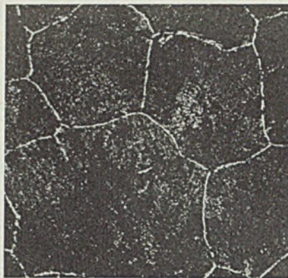
Fig. 15—McQuaid-Ehn grain at 100X of 0.22 silicon, silicon killed heat. Carburized at 1700 degrees Fahr. for 10 hours and treated with Nital etch
