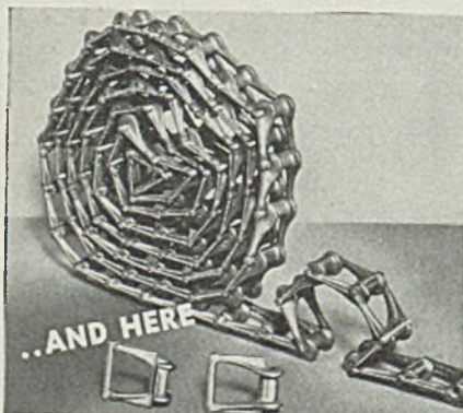
CONVEYOR CHAINS —Important links on continuous pickling equipment—Forged Monel conveyor chain is finding increasing use in pickling service where dependability, high strength and excellent corrosion resistance are required. (Photo courtesy of Steel Improvement & Forge Co., Cleveland, Ohio.)
