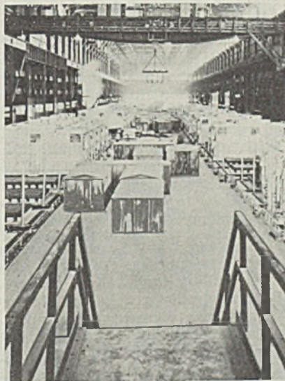
Radiant tube type annealing boxes provide accurate control of heating cycle
