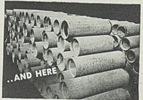
WOOD STAVE PIPE —700 ft. of 12" x 3" shell, wood stave pipe spirally wound with No. 4 B&S Monel wire, was supplied to a large steel company for conveying waste acid from their pickle house. Acid consists of 1 to 7% sulfuric, a small muriatic content at times, water, iron sulfate and small quantities of sand and steel scale. The pipe is covered with a heavy asphalt and sawdust coating and is installed in earth under a concrete floor, the total load on the pipe being about 1500 lbs. per sq. ft. (Photo courtesy of Michigan Pipe Company.)
