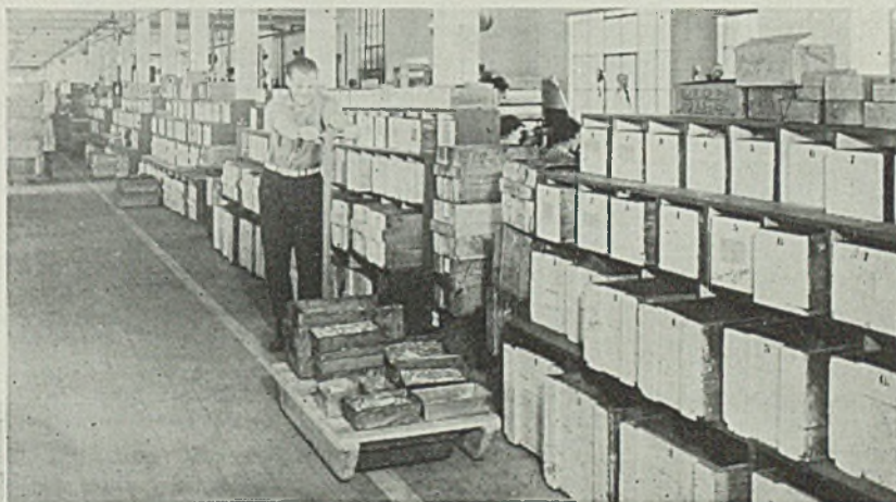
FIG. 1 (left)—View of raw stock storage room. Strip steel is delivered in the form of coils and piled up until needed. A lift truck and skids carry much of the burden in moving material into and out of storage. Fig. 2 (above)—Parts from screw machine and other departments are distributed by lift truck and skids to storage shelves located near assembly lines. Aisles are wide and well marked; rigid rules are enforced to keep them clear for trucking
