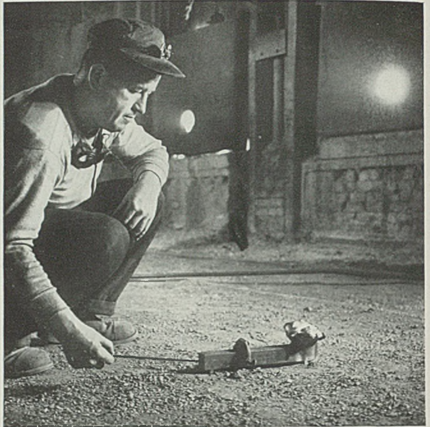
Taking the slag viscosity reading, which forms the basis of VisControl.
