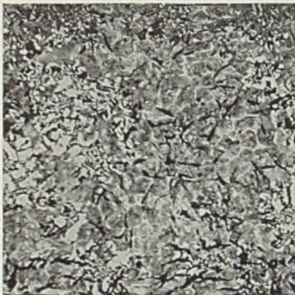
Fig. 1 (Left)—Unenameled casting at 100 diameters showing matrix to be largely lamellar pearlite with white ferrite adjacent to fine network-like graphite nests. Fig. 2 (Right)—Same casting at 500 diameters
