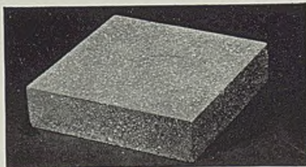
J-M SIL-O-CEL C-3 CONCRETE —An insulating-refractory concrete for temperatures to 1800° F. Recommended for open-hearth flues and below-ground sections of open-hearth regenerators, for bases and lower ring of hot-blast stove, and for furnace bases and doors. C-3 granules furnished in 100-lb. bags; job-mixed with Portland or Lummite cement.
