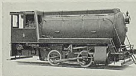
Fireless Steam for Chemical Plant
