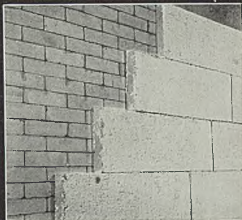
J-M SUPEREX BLOCKS —The most widely used block insulation for temperatures up to 1900°. Economical to install . . . unusually efficient in service. For above-ground sections of open-hearth regenerators, and for hot-blast stoves, mains and bustle pipes, soaking pits, producer gas mains and all types of re-heating and heat-treating furnaces. Furnished 3" to 12" wide; 18" and 36" long; 1" to 4" thick.
