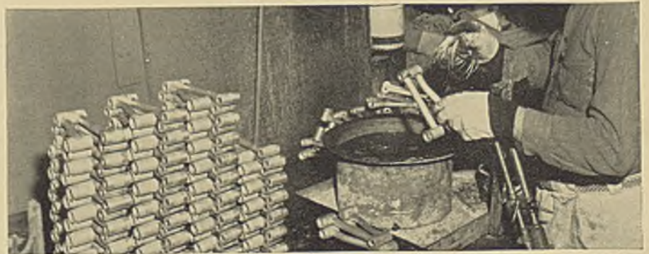
Soldering offers a simple, effective way of producing many brass shapes. When proper care is taken in cleaning, selection and application of flux and solder, strong, efficient joints are readily obtained.
