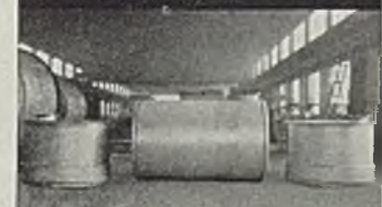
Tanks fabricated of Ingaclad Plate by Leader Iron Works, Inc., Decatur, Ill., for Wilson Laboratories Division of Wilson & Co.
