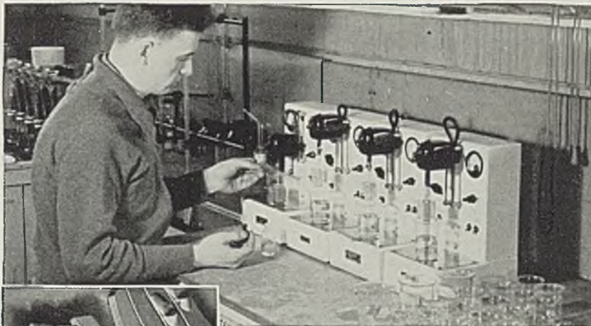
A battery of 4 electro-analyzers determines copper content of the alloy.
