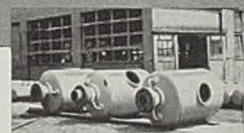
Cereal Cookers fabricated from Ingaclad by Leader Iron Works, Inc., Decatur, Ill.
