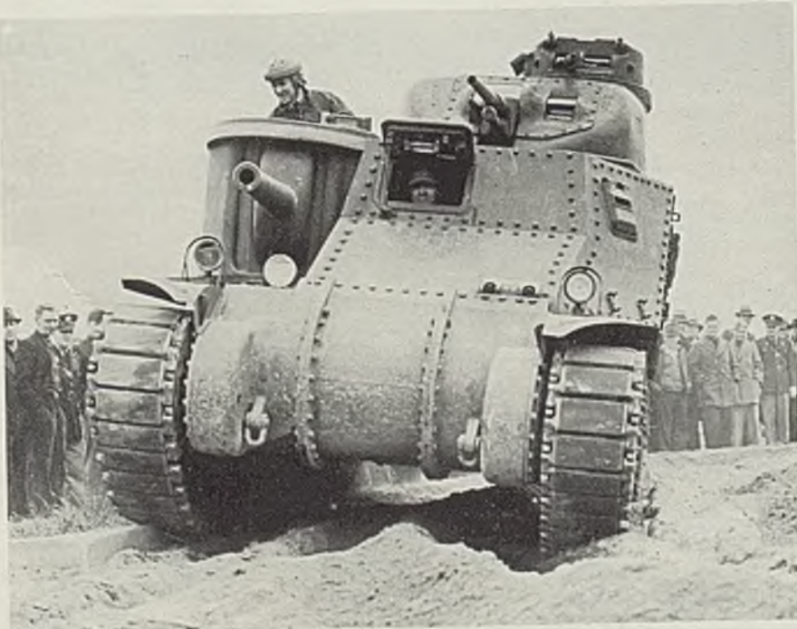
■ Twenty-five-ton medium tank undergoes tests and inspection at the Army's proving grounds at Aberdeen, Md. Tank carries a 75-millimeter field gun, a 37-millimeter antitank, anti-aircraft gun mounted in a power-driven turret, and machine guns. NEA photo
