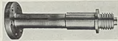
Fig. 3—This is typical of the type of production operation in which depositing a sleeve of metal is not feasible by any other method than by metal spraying because of the flanges or shoulders on each side of shaft portion on which protection is wanted. Shoulder section at right was a 1/8-inch sleeve of sprayed stainless, 25 pounds of metal being applied on this SAE 1045 drop forging for a heavy dredge pump shaft. Sprayed and finish ground in approximately 4.5 hours
