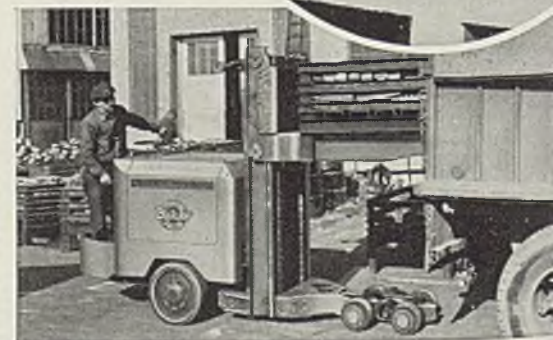
No loading platform required as forged gear racks are loaded into truck for shipment.
