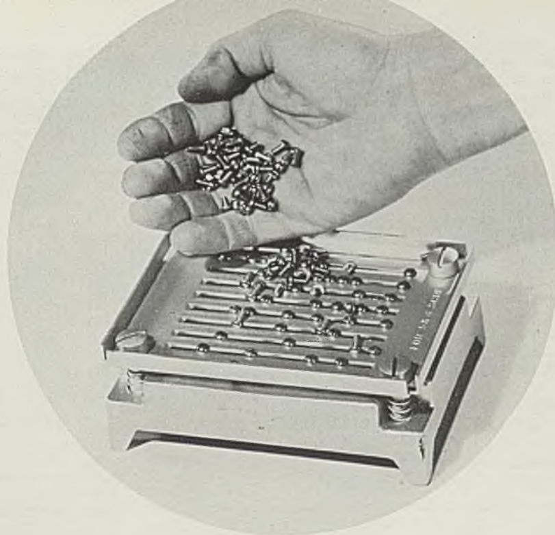
Fig. 1—All types of machine and work screws can be handled by the new device. Here a handful is being dumped into the tray
