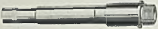
SUPERFINISHED SPINDLE is made of alloy steel with bearing surfaces carburized, hardened, ground and superfinished.
