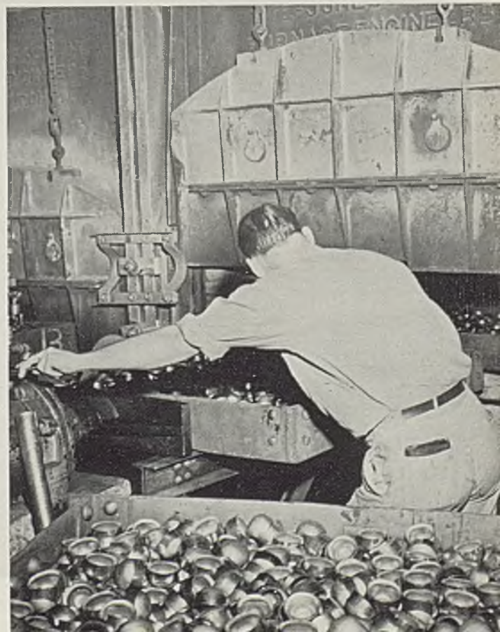
Fig. 2—Here the disk has been cupped and the cups are being annealed to permit further drawing operations at Frankford Arsenal. These will be 75-millimeter cartridge cases eventually. A 75-millimeter gun in action needs 166 per hour. That's almost three each minute
