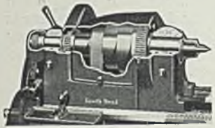
HEADSTOCK. Cutaway view showing integral type bearing and the capillary oiling system.
