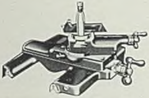
IMPROVED SADDLE and compound rest with adjustable tapered gibs. Cross slide bridge is wide and deep, providing rigid support for the tool rest.
