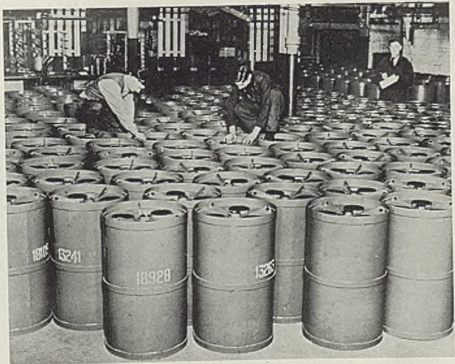
■ They look like ordinary casks but each of these bombs, made in Britain, could blast a submarine out of the water or crush it like an eggshell. The caps are set off by water pressure. NEA photo
