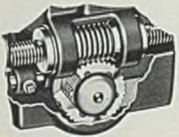
MULTIPLE DISC CLUTCH. Cutaway view shows alternate keyed steel disc construction.
