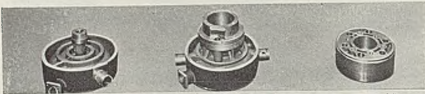
NELOY-MOLYBDENUM STEEL CYLINDER AND PISTON HEAD CASTINGS
