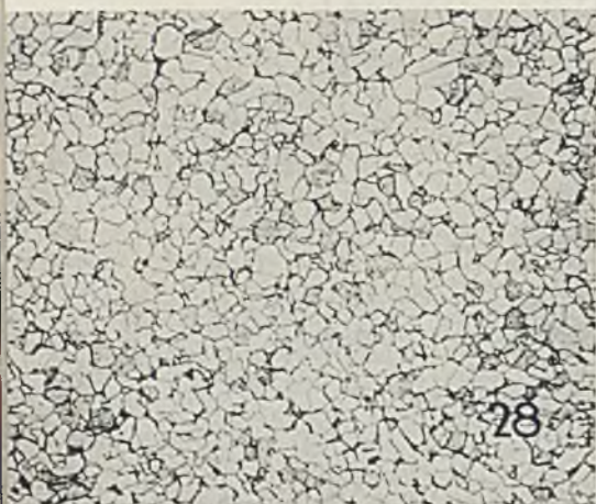
Fig. 28—Bed-cooled strip with microstructure and physical values comparable to normalized material
