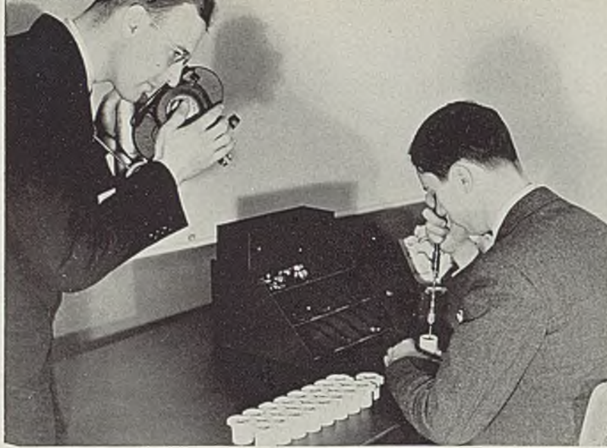
Fig. 3—Here the author, Professor Carson, is adjusting the camera crane to the proper angle to record both vertical and horizontal movements of the operator
