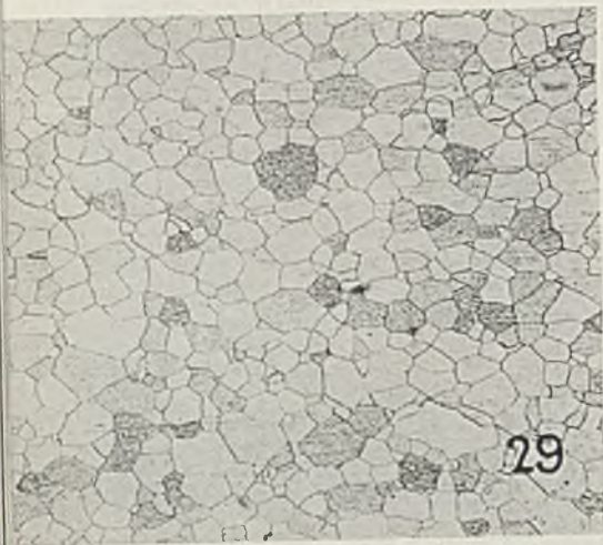
Fig. 29—Same steel as shown in Fig. 28 but coiled 300 feet from mill at 1320 degrees Fahr.
