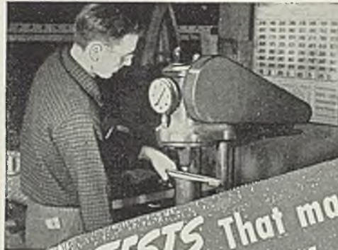
Testing Hardness with Brinell Machine
