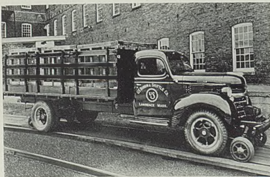
■ Combination of interplant rail hauling and outside road duty is provided by this Dodge 1 1/2-ton truck at the U. S. Bobbin & Shuttle Co., Lawrence, Mass. Rail service is provided by a "railer" pilot wheel attachment, front and rear, the rear tires still providing the power despite the fact the pilot wheels carry a part of the load. The pilot wheels are raised automatically for conventional road service
