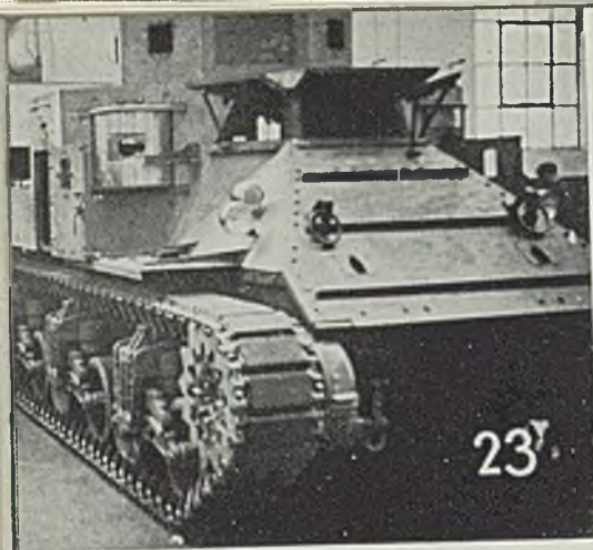
Fig. 23—Tune-up station at end of the assembly line where engines are started and tuned up in preparation for the 75-mile road test. The tank shown here is a larger unit than the others in this series of illustrations
