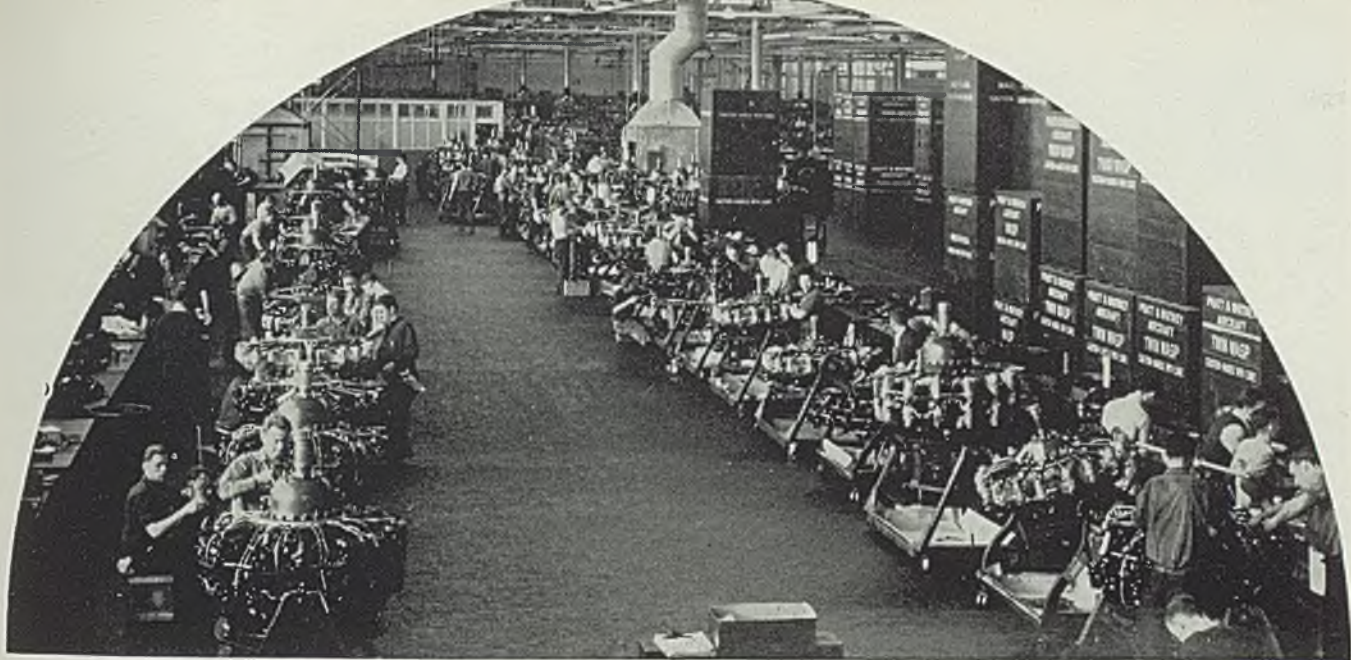
Part of packing and shipping department in new engine assembly building at Pratt & Whitney Aircraft. Here final adjustments are made on engines prior to shipping preparations
