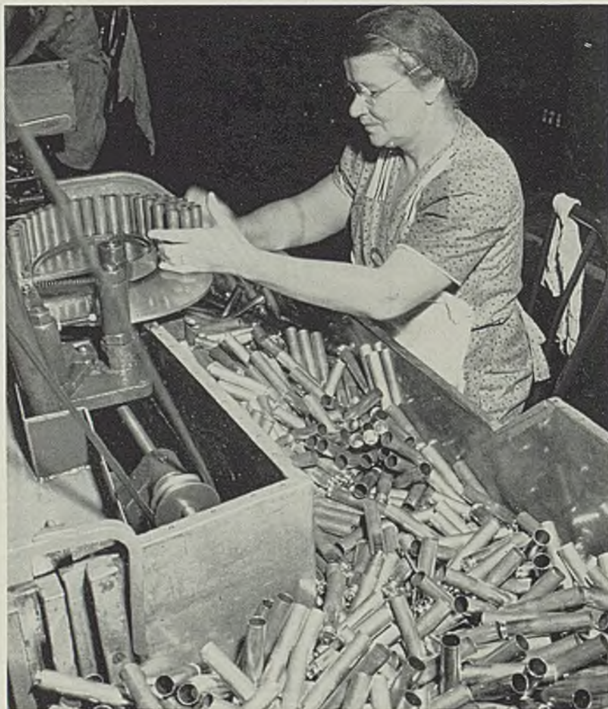
Fig. 3—Many women as well as men are speeding munitions work. Here a woman is feeding 0.50 caliber cartridge cases into a machine which will taper them, part of the process of making antitank ammunition at Frankford Arsenal, Philadelphia. Figs. 3 and 4 from National Defense Advisory Commission, photos by Palmer
