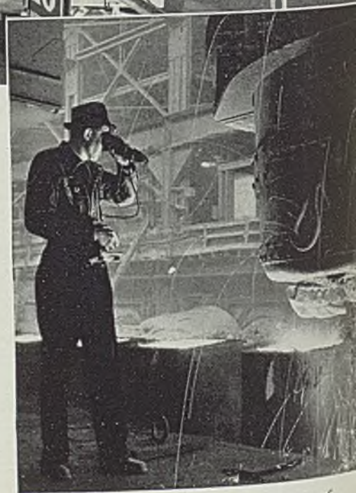
Skilled eyes take the temperature of molten steel with an optical pyrometer.
