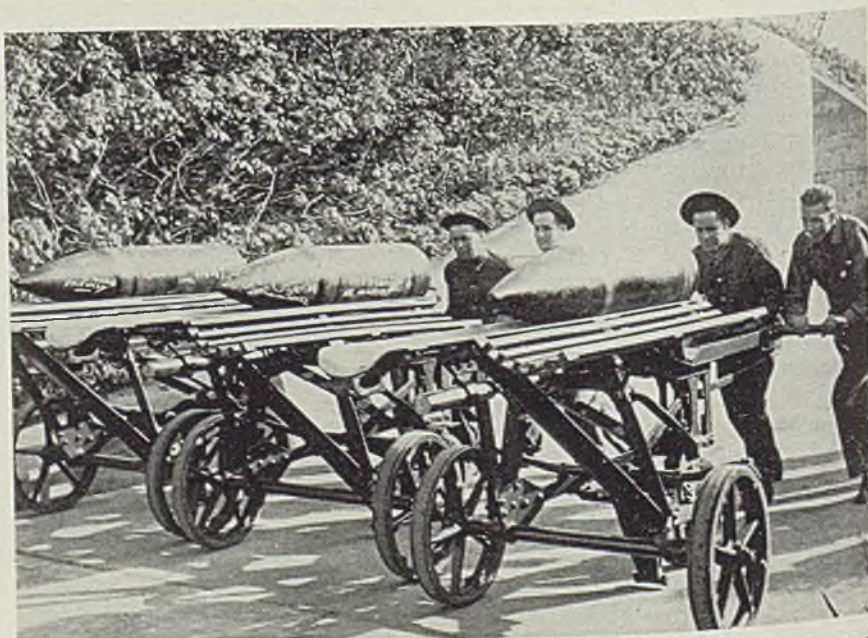
■ "Food" for the 12-guns at Ft. Hancock, N. J., are 1000-pound projectiles, which the gun crews move easily in carriages built of light structurals. NEA photo
