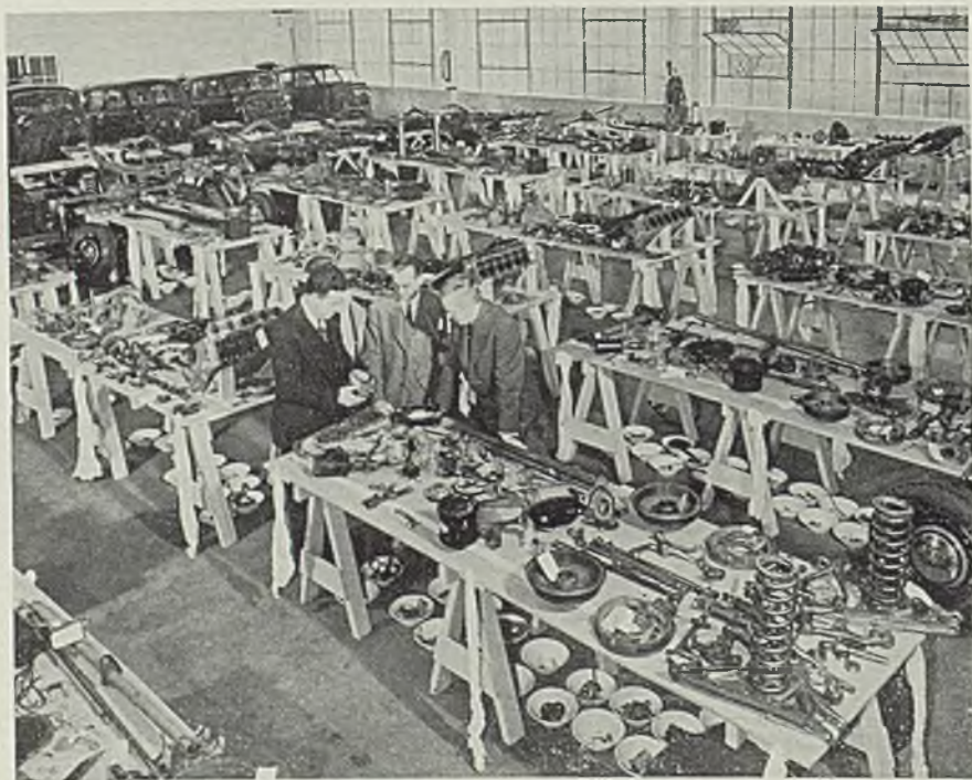
■ Here are parts of 15 different 1941 models laid out for inspection after 25,000-mile test runs of the cars at General Motors' proving grounds, Milford, Mich. E. E. Wilson, director of the grounds; P. A. Collins, Chevrolet experimental engineer; and J. G. Wood, assistant Chevrolet chief engineer, are inspecting some of the parts. Six weeks was required just to disassemble the cars and to clean and arrange the parts for comparison. Later, all cars will be reassembled and tested further
