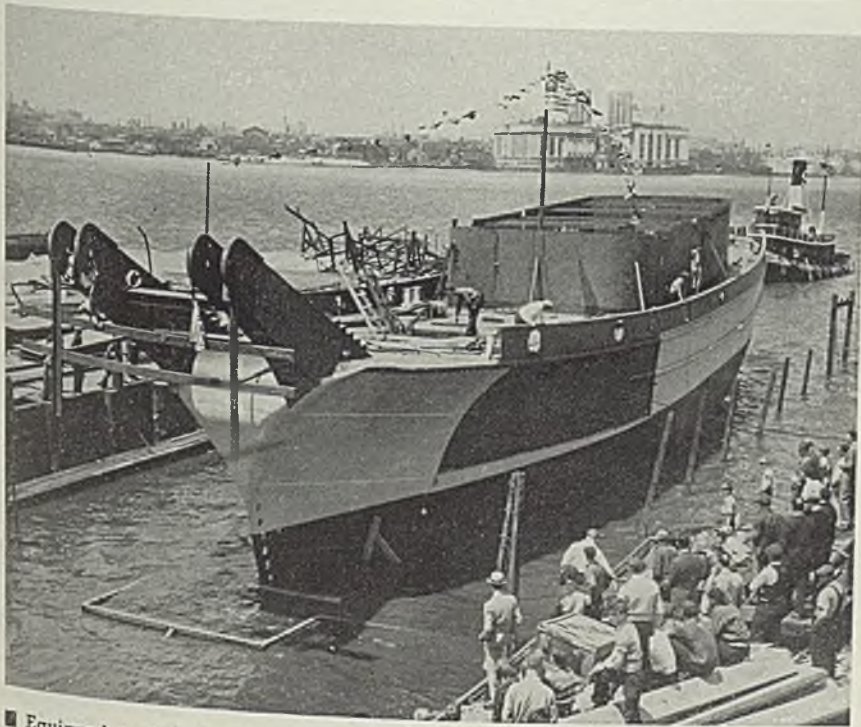
Equipped to handle heavy steel cable nets which may be stretched across harbor entrances and navigable rivers as ant submarine protection, the U. S. S. TEABERRY , 700-ton net tender, was launched last week at the John H. Mathis & Co. yard at Camden, N. J. It is the first net tender to be built on the Atlantic seaboard and will be one of a fleet of 32 to be completed soon. NEA photo
