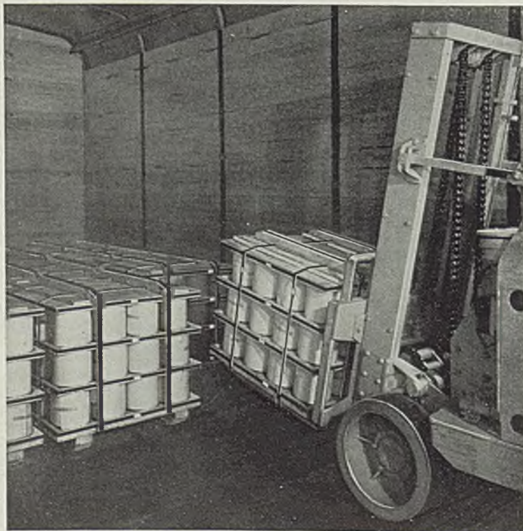
Fig. 1—Steel strapping spools of wire onto wooden pallets as shown here affords a 46 per cent saving in cost and reduction of 95 pounds in tare weight
