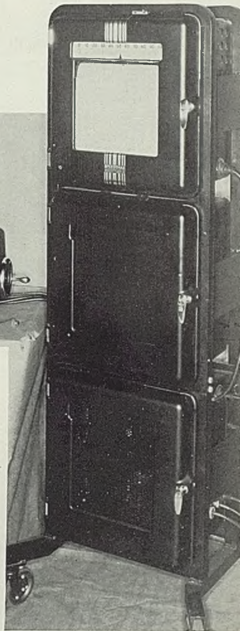
Fig. 1—Leeds & Northrup's new recording Microphotometer: The setup consists of a plate-scanning unit, shown at left, above, and a Speedomax recorder, at right
