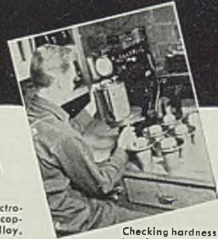
Checking hardness of parts by Rockwell machine.
