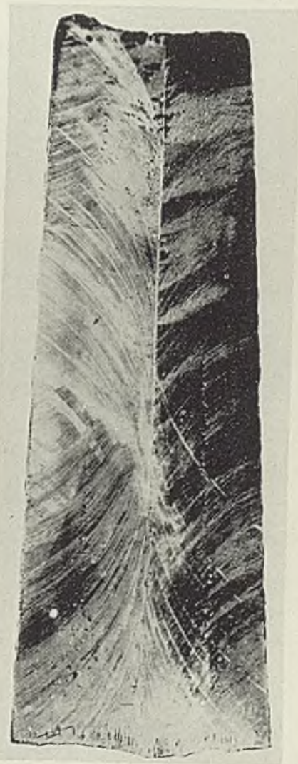
Fig. 1—Ingot free from skinholes on the sides, but with a few scattered over the bottom
