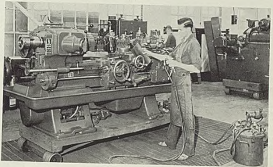
Fig. 7—Close-up of machine over the down-draft spray pit, which permits spray painting and slushing of complete machines "right out in the open". All fumes and drifting spray are sucked down into the pit and the work is done without the slightest inconvenience to others working in the near vicinity. Spray gun application of rust-preventing "slushing compound" to bright parts—as depicted here—is a new and very effective method
