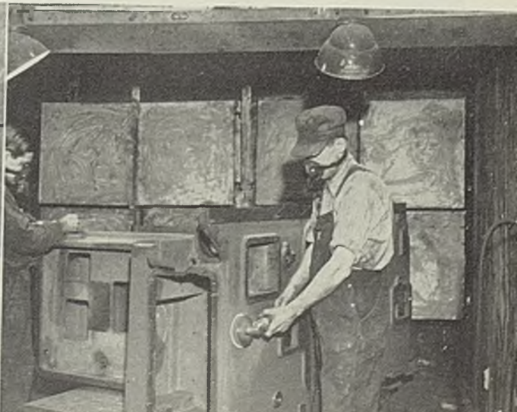
Fig. 4—Sanding down filler coat on frame casting, using rotary disk sanders made from converted air drills. Hand sanding is resorted to only in inaccessible pockets and corners. This work is done in a suction ventilated booth and lead-free fillers are used, respirators being worn at all times as an extra measure of health protection
