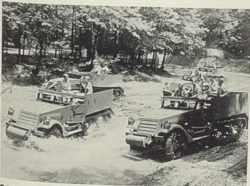
Fully manned, and with machine guns mounted, five armored half-trac reconnaissance vehicles, first of 5308 now under production at White Motor Co., Cleveland, demonstrate their ability to negotiate difficult terrain by dashing through mud and water nearly 3 feet deep
