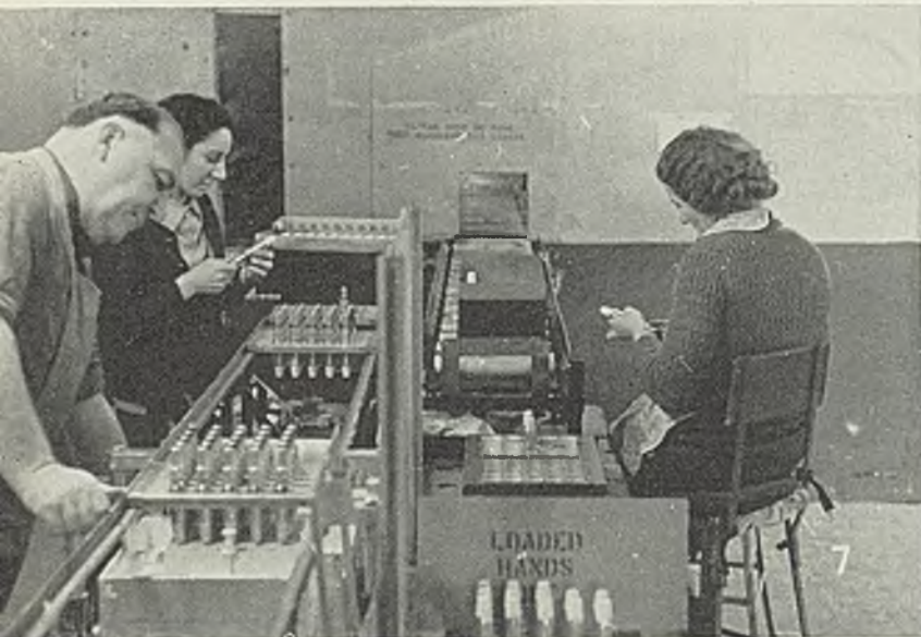
Fig. 7—Here fuzes have passed through many preliminary steps in assembly and are having their heads painted by dipping inverted into the paint. Note that fuzes are handled through assembly operations in racks of 25 units. In this portion of line, these racks are moved down the line between rails spaced the correct distance apart. Dipping is done by lowering a movable section of track over the paint tank. This station is also shown in immediate foreground of Fig. 2. After being inspected and set in racks in boxes, the fuzes are passed through the small opening in the wall into the
