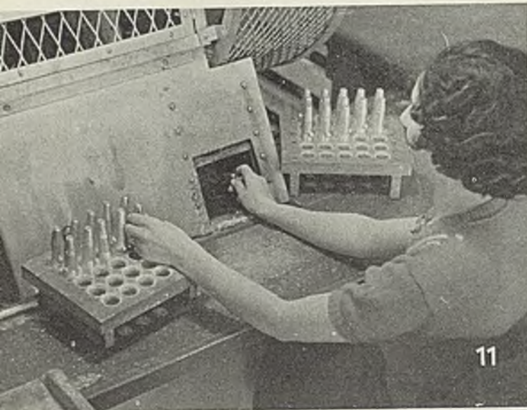
Fig. 11—This eccentric press used to crimp the fuzes is heavily barricaded to protect the operator. The small opening through which she inserts work has a sliding door which falls as the press starts the crimping operation, thus completely protecting the operator. Instead of a positive drive, a spring drive on the door prevents any injury to the operator's fingers if they are not clear when the door closes
