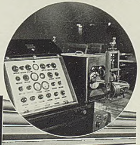
Magnetic testing finds the slightest hidden flaw.
