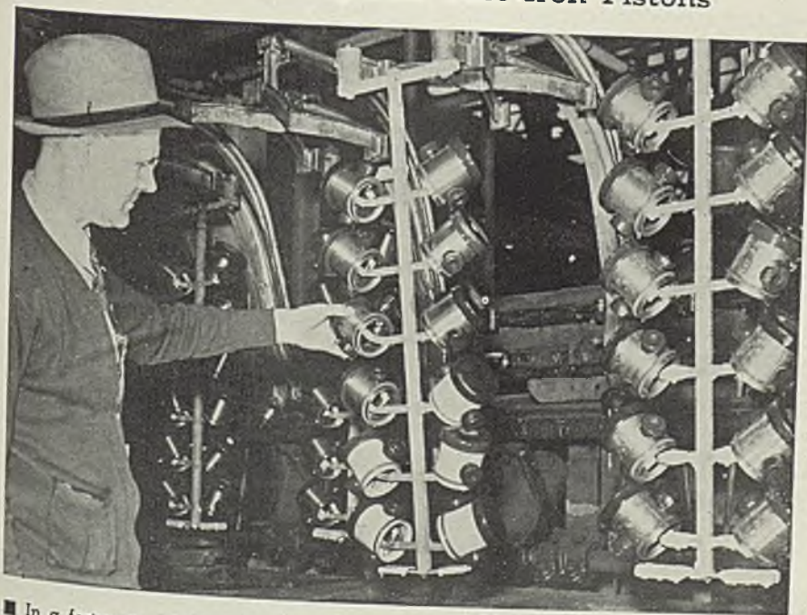
■ In a fortunate position by virtue of having always used cast iron pistons, Pontiac Motor Division, Pontiac, Mich., anticipates no difficulties from material scarcity on this score. Here are racks of machined iron pistons about to be lowered into electroplating bath which plates a layer of soft bearing metal on the skirts. Rubber caps over top and ring grooves keep the plating off those sections. Lower five pistons on the center rack have received plating
