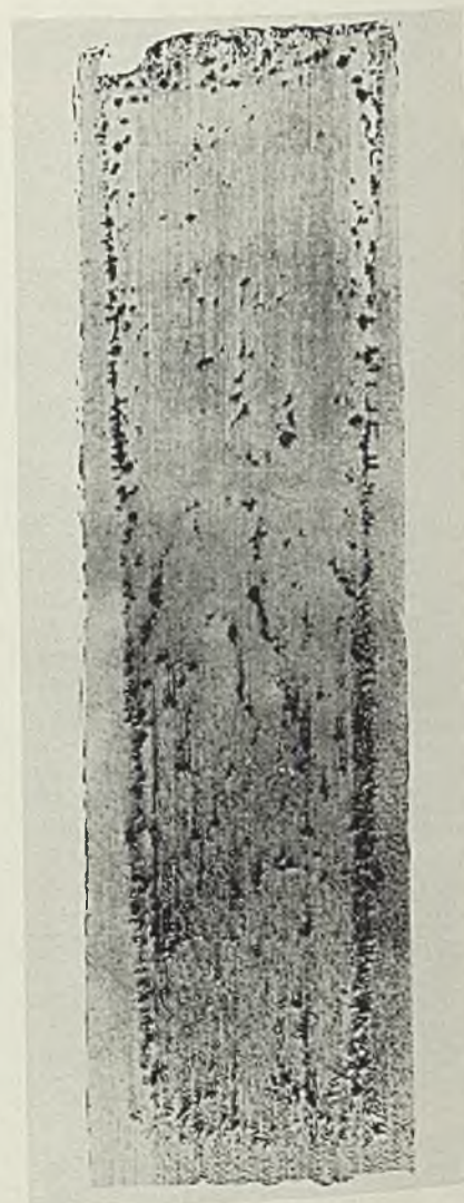
Fig. 3—Excellent quality of rimmed steel ingot free from skinholes
