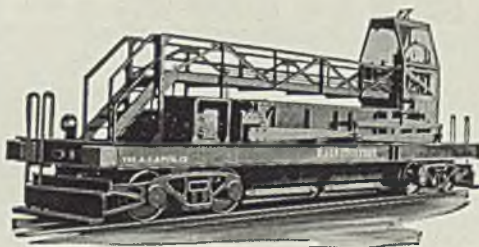
20 Ton — Double Compartment Scale Car. Journals provided with self aligning anti-friction bearings. Equipped with Atlas Indicator and Recorder.
