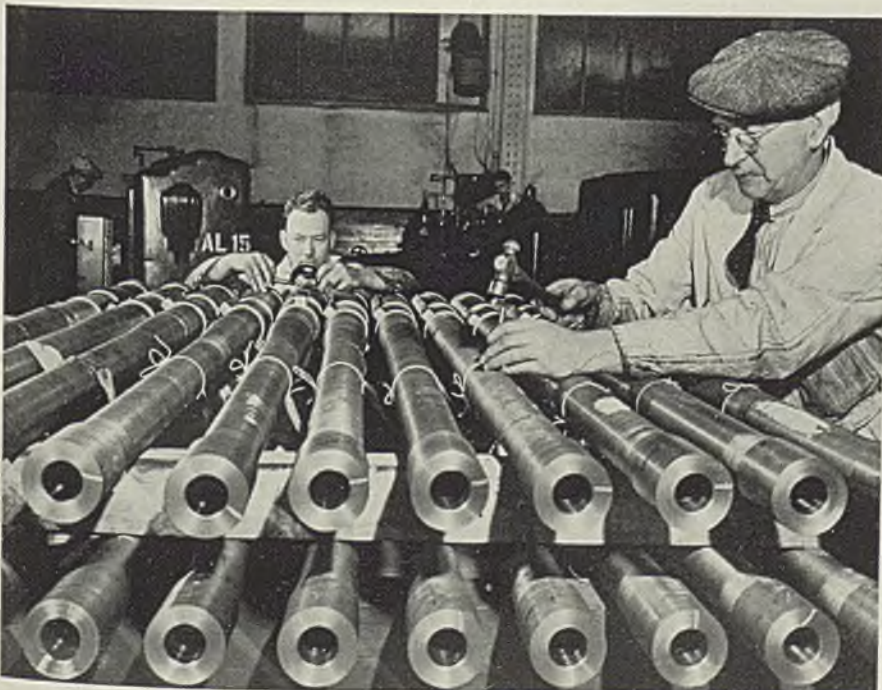
■ More than 1000 operations are required in the manufacture of a new 2-pounder anti-tank gun now in production in Canada. This photo shows a line of the 2-pounder gun barrels being inspected. Craftsman at right is a veteran armament worker from England. First consignment of these guns already has been shipped to United Kingdom. NEA photo, passed by censor
