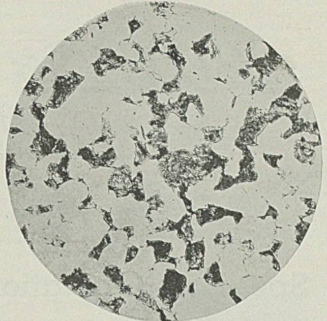
L EFT view shows direct quenched core structure, X500, while photomicrograph at right shows the new steel in the normalized state at 1700 degrees Fahr. at the same magnification
