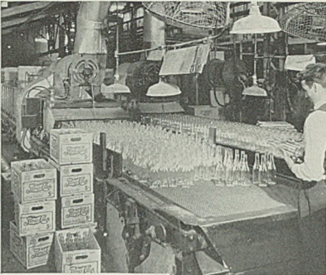
Above is shown Cambridge Interwoven belt conveying bottles through a glass annealing lehr.
