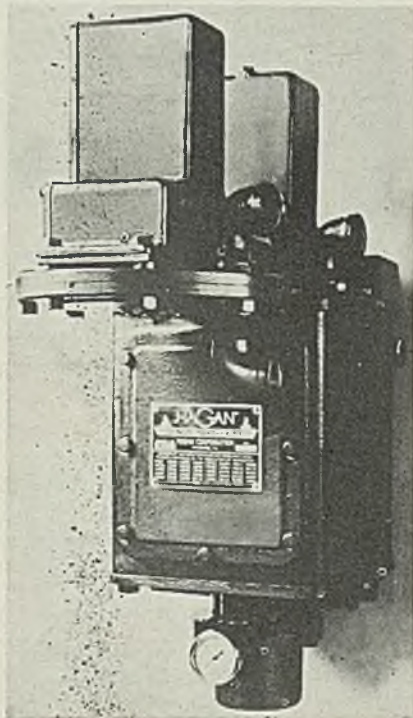
Hagan oil-operated regulator controls ratio between pressures or differentials
