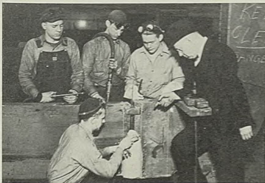
TOM JONES, welding shop foreman at the South works, shows trade apprentices how to prepare a thermit weld on a beam mill manipulator bar. Art Algrim is making the wax pattern, Lyle Burge is waiting to trim it with the knife, while Arnie Jensen will use the cutting torch to fit a flask around the pattern. Bob Price will later pack it with sand with the air hammer
