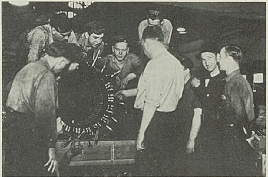
APPRENTICES enrolled in the training course are given a comprehensive view of the entire plant through work in many different departments. Here is a group working in the electrical construction division learning methods of building up motor windings
