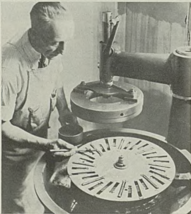
INJECTION pump plungers require 25 separate machining operations, five of which are performed on the automatic machine at the right. In the foreground is a group of "semiformed" plungers which in the finished state require extreme accuracy
