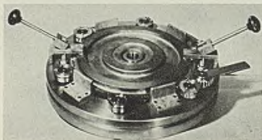
FLYWHEEL assemblies can be finished to advantage in the Garrison chuck
