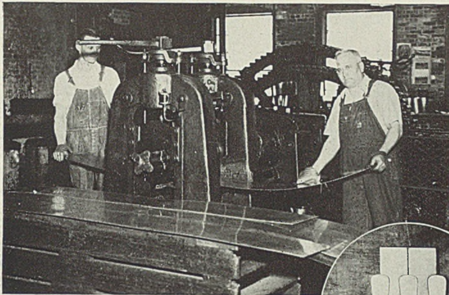
F IG. 3 (left) shows 2-high mill with 12-inch rolls having 16-inch face used in rolling silver for flatware. Fig. 4 (inset) shows teaspoon blanks so cut as to prevent wastage of metal. Fig. 5 (below) shows the "grading" operation, performed in a miniature rolling mill with one roll off center; this operation, used in forming flatware for teaspoons, leaves the stock thicker at the center than at the ends. Fig. 6 (at bottom) shows the "striking" operation, in a drop hammer, by which beautiful designs are formed on silver spoons and forks
