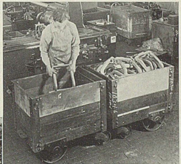
FIG. 1 (below)— Electric platform truck carrying pans of small parts and drawing train of five special box trailers. Note the wide and well defined aisles; floors are of impregnated wood block
