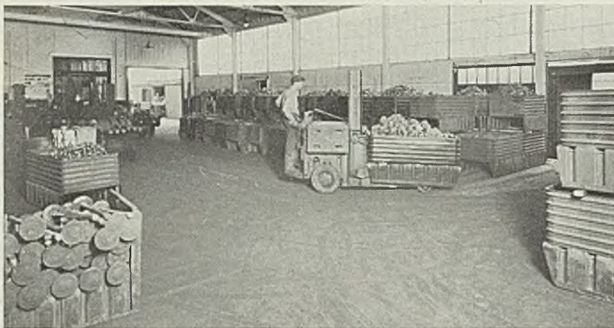
F LEXIBILITY of the skid-and-box system is shown to good advantage in the shipping department
