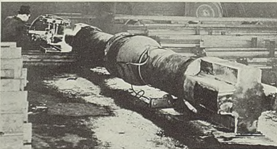
Flame hardening is considered the only practicable method for hardening the wobbler pads on this 9-ton spindle
