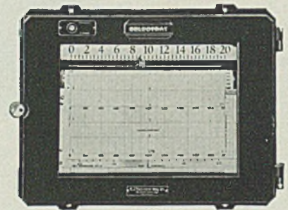
Tag "Celectray" recording potentiometer has a sensitive mirror galvanometer as the primary controlling element
