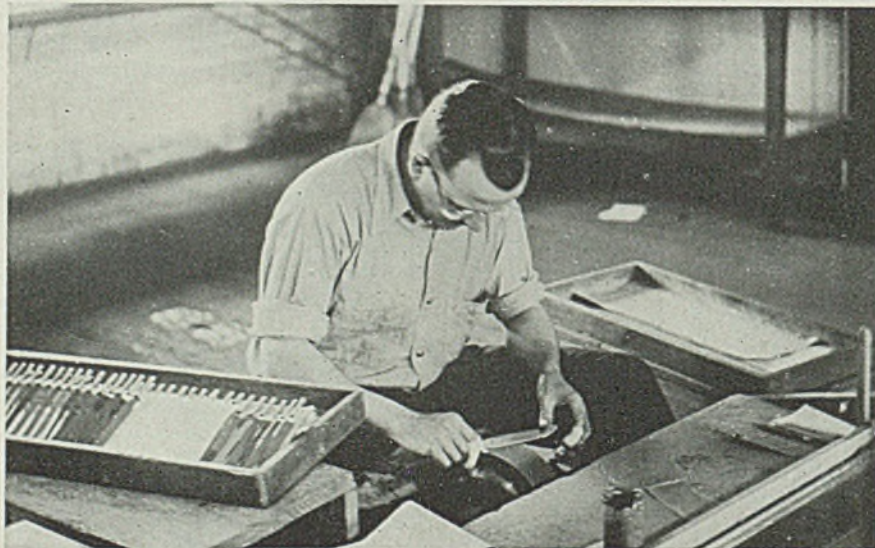
FIG. 9—Edging or sharpening the I blades is done by hand on an alundum wheel operating at 2500 revolutions per minute
