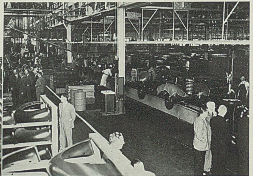
FIG. 7 (above)—This is a view of the chassis assembly line. Electric tools are suspended from an overhead feedrail as shown at the right. Fig. 8 (left)—After bodies are attached to the chassis, the cars move along a floor level conveyor for the final assembly operations. This is followed by inspection and test
