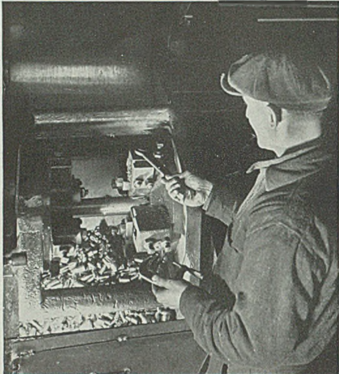
Turning a bar in precision machinery to produce J&L Turned and Ground Shafting. After turning, the bar is ground to final dimension, with extreme accuracy.
