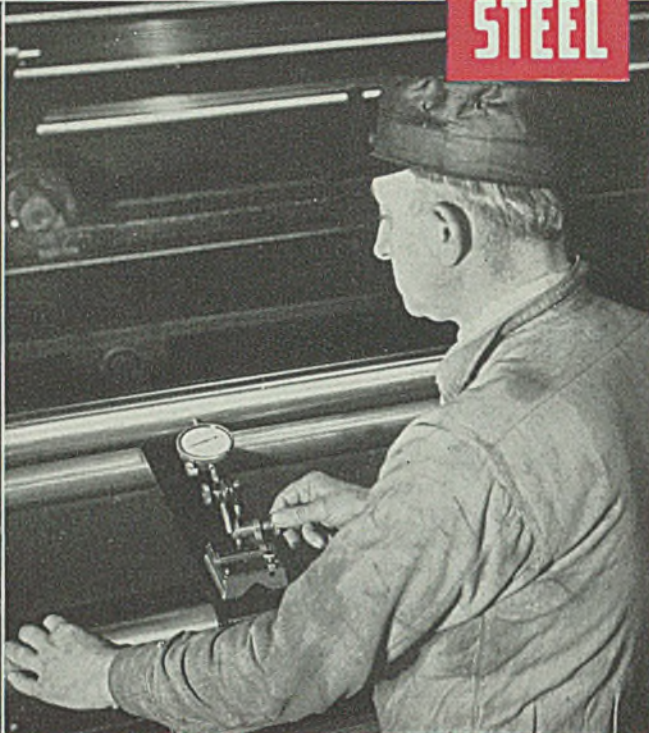
J&L Turned and Ground Shafting is straightened by an exclusive J&L process and must pass a rigid inspection for straightness.
