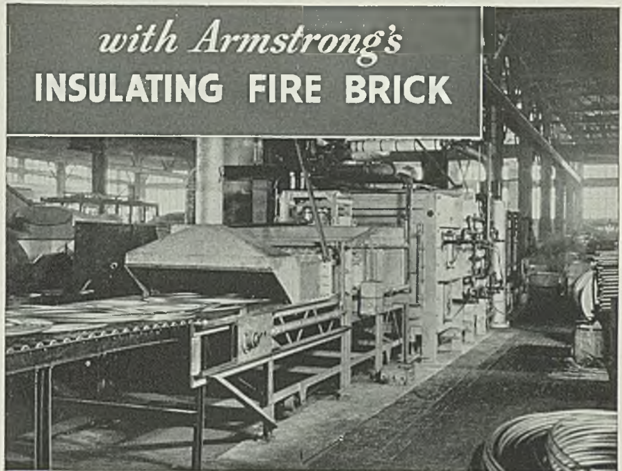
Armstrong's EF-22 Insulating Fire Brick assure more efficient operation of this modern furnace for coil brass work. The furnace is gas fired, of the conveyor type.
