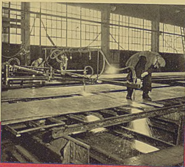
Three views of the Airco No. 20 Travograph showing the extremely wide areas over which this machine can operate.
