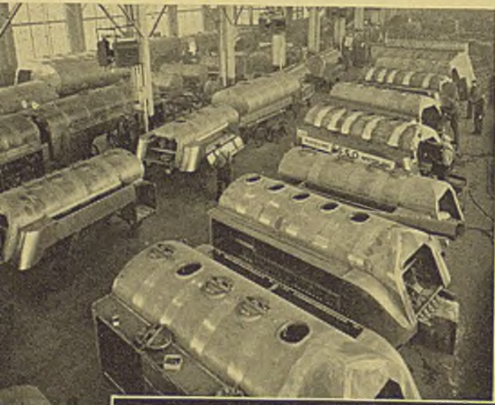
Below, finishing department in a plant making tank trucks. These include milk and gasoline trucks, all welded
