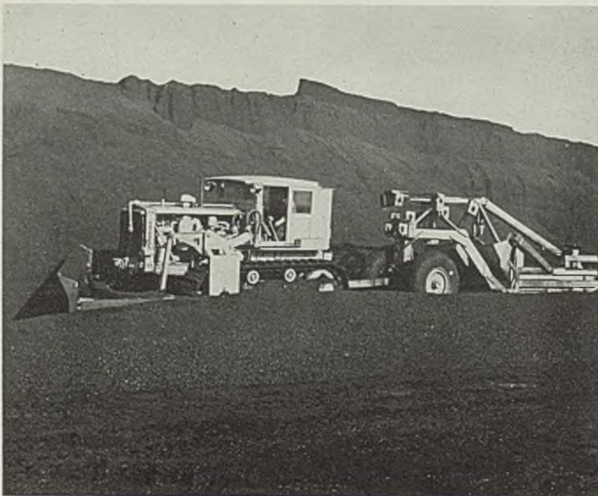
Fig. 1—A modern heating and air-conditioning device has been installed in this iron horse for the comfort and health of the operator. Hauling a carryall and shoving a bulldozer, this unit handles an average of 130 tons of coal per hour
