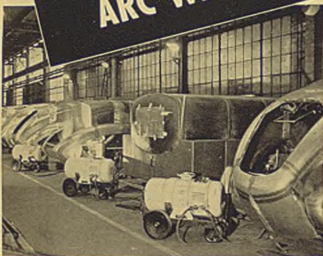
Here several Wilson "Hornets"* — newest of the line of electric welders that make the arc behave — are being used to fabricate garbage disposal trucks for the City of New York.
