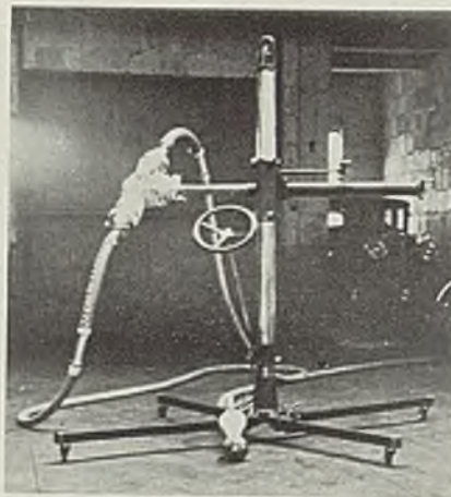
Fig. 1—Shock and rayproof x-ray tube mounted on flexible stand
