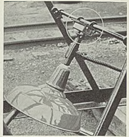
Fig. 4—Mounted on boom of a drag shovel, much lamp breakage was encountered until the vibration was insulated from the lamps by the mountings shown
