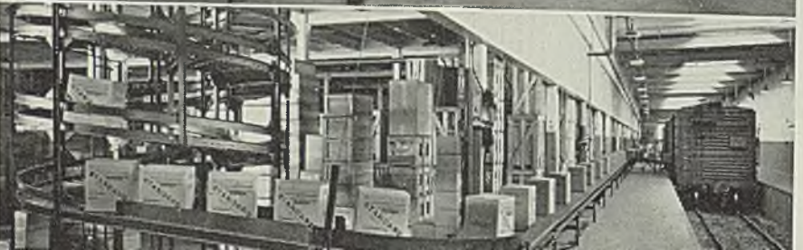
Fig. 8. (Next to bottom)—A spiral chute takes products from second floor
