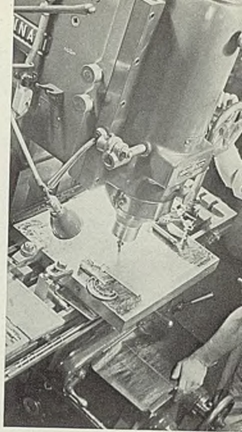
Tool engineering problem of accurately spacing precision bored holes in bolster plate, is solved in this case by Cincinnati vertical, dial-type milling machine equipped to use precision measuring rods in conjunction with dial gage reading in "tenths"
