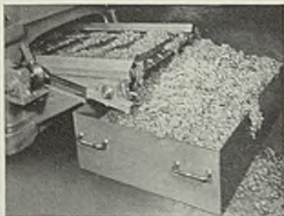
Cone Automatic Chip Remover used on the machine described above.
