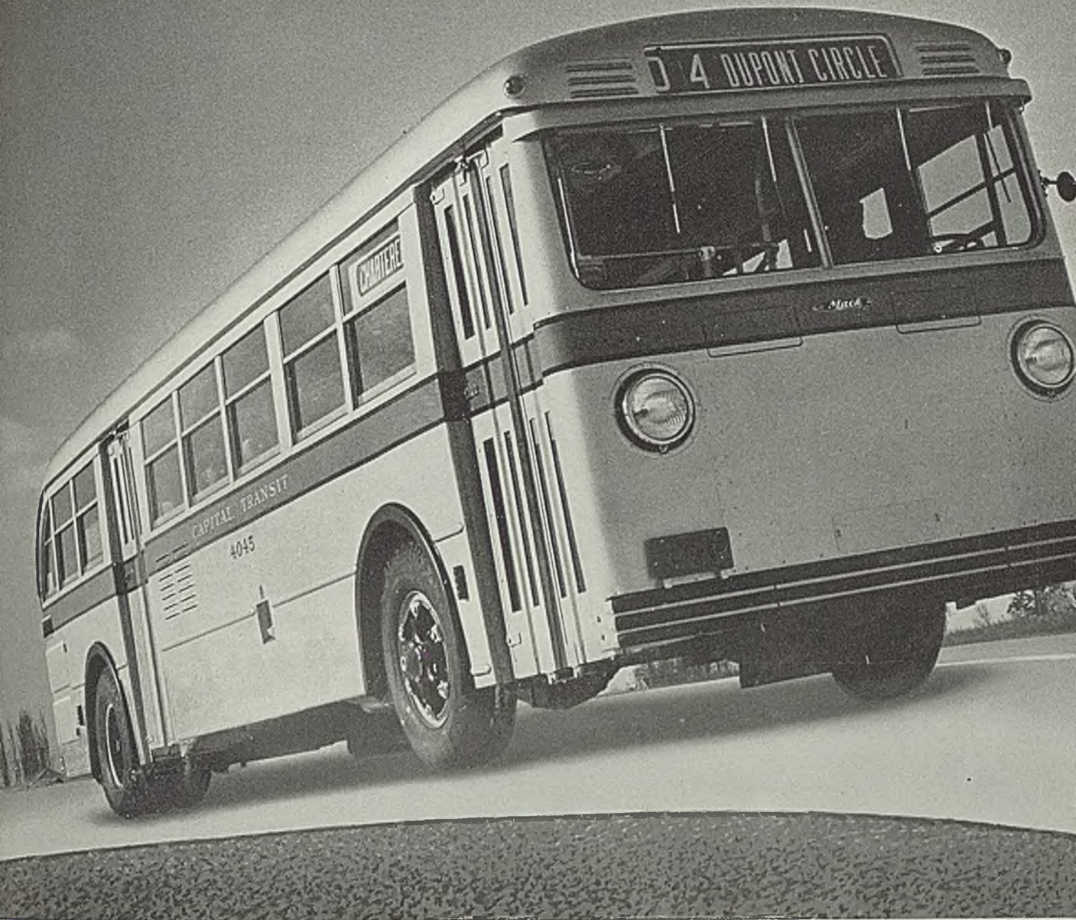
41-Passenger Mack Bus with structural members of "A.W." DYN-EL high strength steel.
