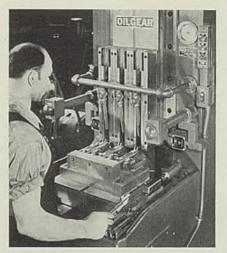
Fig. 1—This Oilgear broaching machine with special tools and quick-operating work-holding fixture enables one operator to machine both sides of 600 rifle receivers per hour
