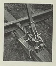
maintain firm grip on ties of various sizes without screws, clamps, etc., and without damaging tie. Device is sufficiently light for han-
