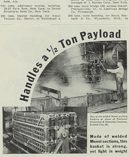
How you can boost your payload . . . and thereby cut production costs . . . is well illustrated by this lightweight basket of welded Monel. One of ten baskets used for pickling stamped steel hollow ware before enameling, it weighs 400 lbs., is 30 inches high, 30 inches wide, and 6 feet long.
