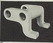
Easy to use, Genex Electrodes are often employed in making small units to replace castings, such as this one built by The Darr Company, Denver.
