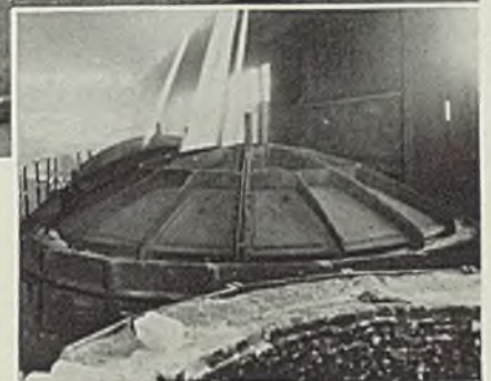
● Inside and outside views of 12-ft. annealing furnace cover of this steel works, showing Refractory Concrete lining, made with Lumnite. This job was done quickly and easily. No joints to leak heat. Plenty of strength to resist the hard knocks these covers get.
