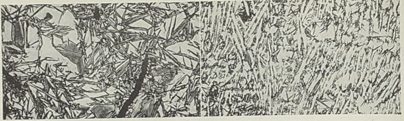
Fig. 3A. (Left)—Coarse martensitic structure resulting from treatment at excessive temperature. Fig. 3B. (Right)—Excessive temperatures produced this structure in the case near treated surface. Both at 500 diameters
