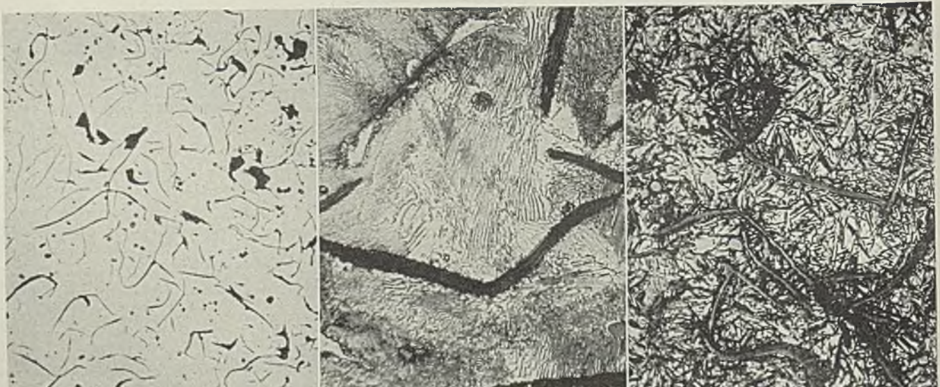
Fig. 1A. (Left)—Unetched view showing graphite distribution at 100 diameters. Fig. 1B. (Center)—Pearlitic base material. Fig. 1C. (Right)—Martensitic structure of case immediately below surface, both at 500 diameters
