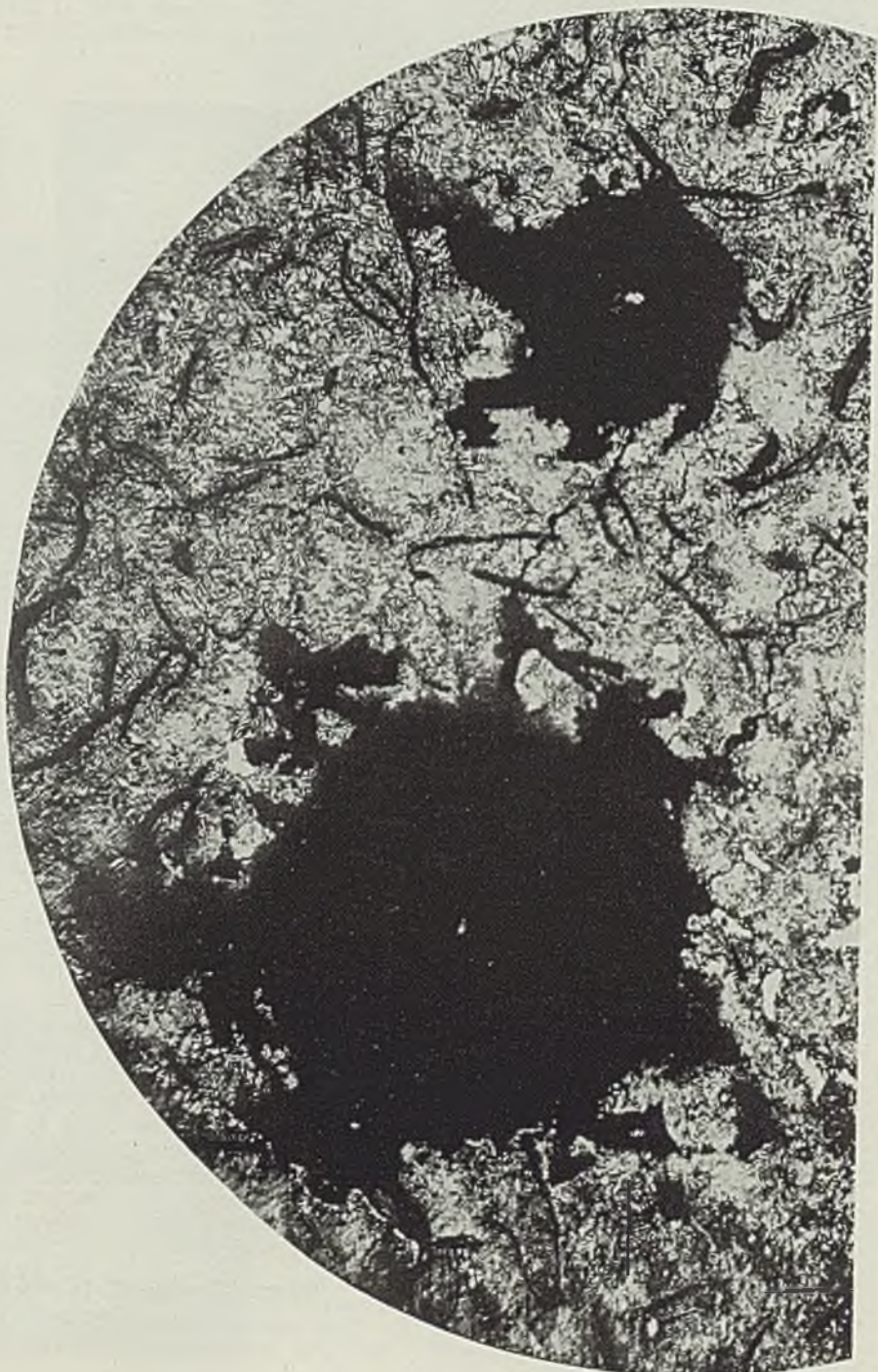
Fig. 6—This illustrates difficulties encountered in penetration testing gray cast iron. Note crumbling even on edge of small indentation made with 30-kilogram load
