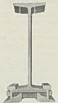
Shepard Track consisting of two special analysis T-rails clamped to the bottom flange of a standard I-beam insures a smooth, hard, long-wearing track for monorail hoists.
