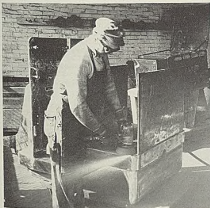
Fig. 4. (Right)—Welding heavy plate to make frame for a power truck. Operator is using electric arc
