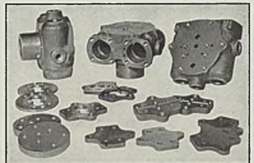
Group of parts ground on the Blanchard No. 18 shown at the left.
