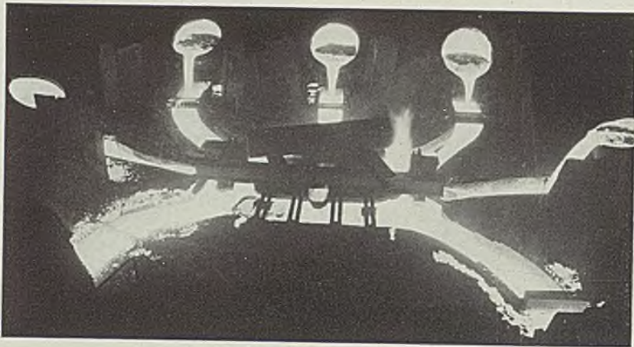
■ Seven ladles were employed recently in casting a large ingot mold at the Bethlehem, Pa., plant of Bethlehem Steel Co. The casting weighed 350,000 pounds and was poured in one minute and forty seconds
