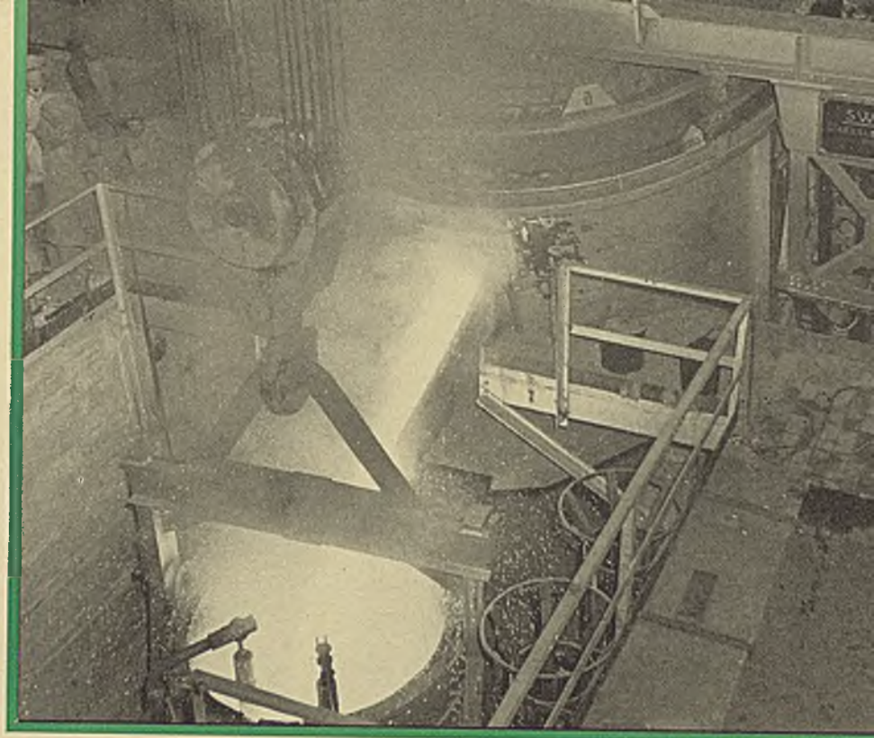
Heat of steel being poured from one of the 25-ton electric furnaces. Casting pit serves both furnaces
