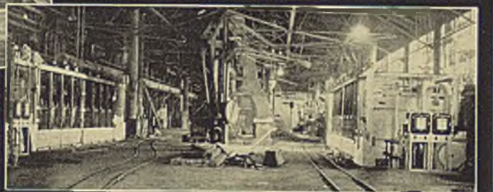
Group of hammer furnaces for alloy steel.
