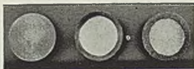
Cross-sectional view of three tie-rods after a 12-month test in well-known steel sheet mill. Monel (left) is uniform through its whole diameter. The other two rods, while still unchanged in diameter, are weakened by a change in their metal structure brought about by corrosion.
