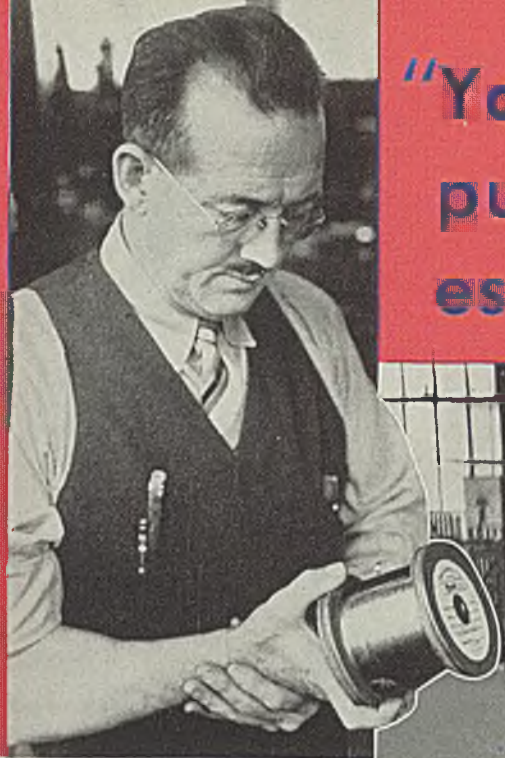
The finished product: Spool of ribbon-type Chromel, bright annealed.
