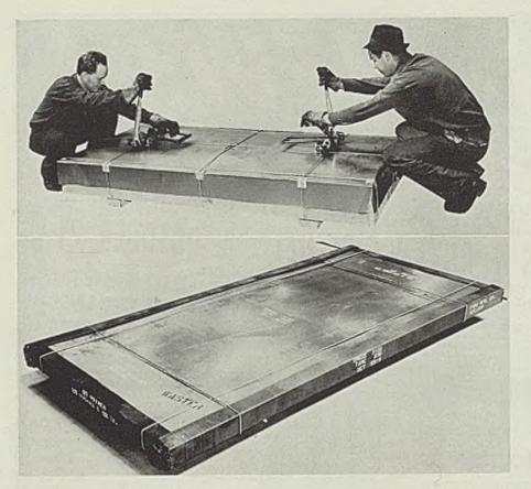
Fig. 2. (Upper)—Large steel sheets are protected by first wrapping with waterproof paper, covering with hot tar, adding sheet metal cover and tying to skids. Fig. 3. (Lower)—These 20-gage sheets, 43 x 92 inches, have added protection provided for the corners by 16-gage steel rails, clinched tightly at all corners and tied into the package
