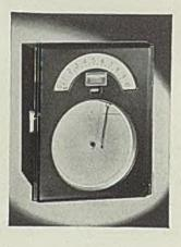
easily adjusted by changing a calibrating weight, has a 12-inch evenly graduated chart and is furnished with any combination of indicator, recorder and cyclometer integrator.
