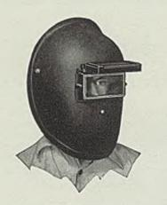
and weighs only 15 ounces complete with lens and holder. Helmet is of lift-front type that gives operator a dense lens in the outer holder and a clear lens or less dense lens set in the inner holder. The inner and outer frames have concealed spring hinges which allow the outer holder to be raised or lowered in accurate positions. Holder is interchangeable and is held in position by two screws.
