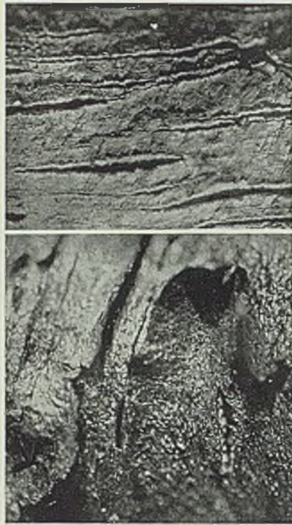
Fig. 11. (Above)—Photomicrograph of hair-line seams. X4½. Fig. 12. (Below)—Photomicrograph of corner defect. X4½
