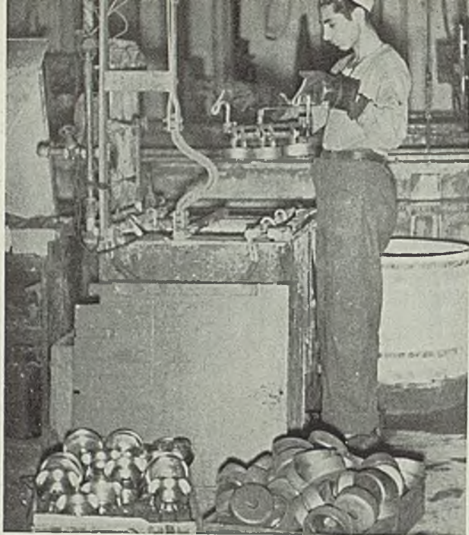
Fig. 1. (Left)—A typical tank installation for electro-polishing stainless. Tank has heating and cooling elements for temperature control, employs copper racks to hold work. Courtesy Phillip Sievering Inc., 199 Lafayette street, New York. Fig. 2. (Right)—Two 18-8 stainless springs at top show appearance before and after electro-polishing. One half of the spring in the center has been treated. Bottom shows 18-8 rivets before and after treatment
