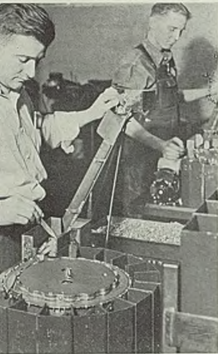
Fig. 2. (Left)—This machine can be set to throw out either round head or flat head rivets, sorting the others according to length in the 13 bins around periphery of wheel
