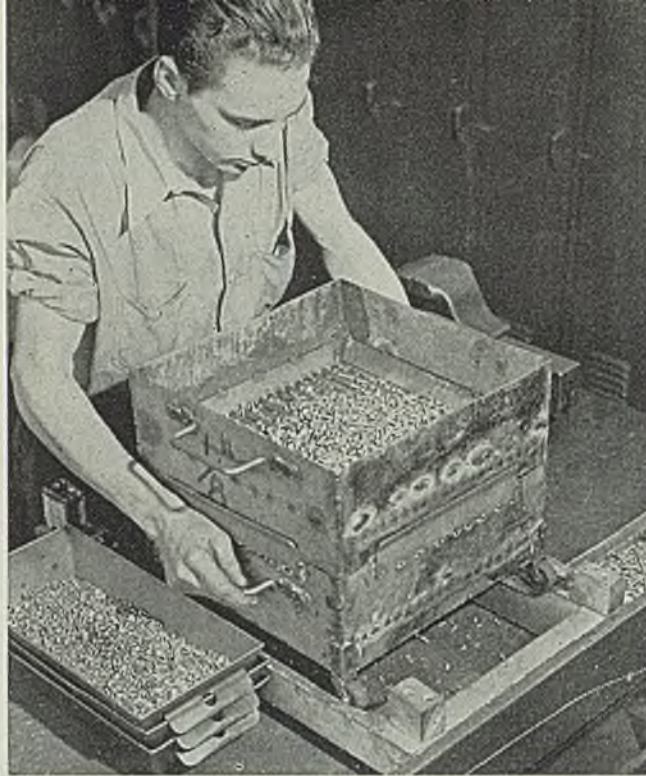
Fig. 1. (Left)—First step in sorting rivets after separation from other sweepings is to sift them according to diameter using sifters shown here
