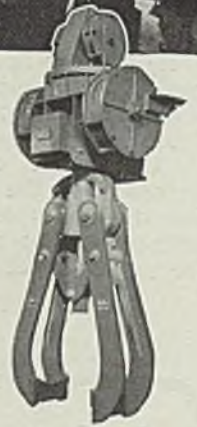
Type FHP welds stand the gaff in these stripping tongs made by Shaw-Box Crane & Hoist Co.
