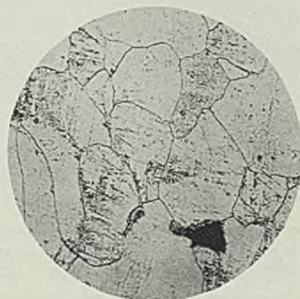
Fig. 13. (Left)—Photomicrograph of chip taken from a slab. X100. Fig. 14. (Center)—Photomicrograph of grain structure adjacent to area under chip shown in Fig. 13. X100. Fig. 15—Example of hair-line seams and strain-lines. X15
