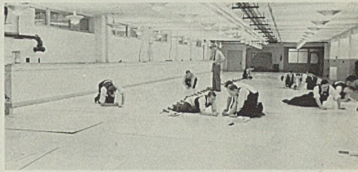
THE LOFT. Borrowed from the shipbuilding industry is this idea—a raised floor on which whole airplanes may be laid out in full size. Then come stress analyst engineers to fill in details. Drawings then are transferred to the metal sheets, production started immediately
