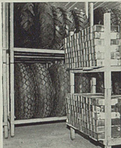
Fig. 10—Racks designed especially for maximum flexibility in handling and storage work. Pins at lower ends of vertical posts make nesting easy
