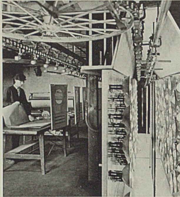
Fig. 1—Certain pieces bake in 8½ minutes in oven at right, emerge to be wrapped at stations on left. Pusher used on this portion of conveyor
