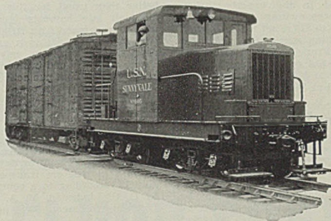
45 Ton Locomotive especially suitable for economical interplant switching service.
