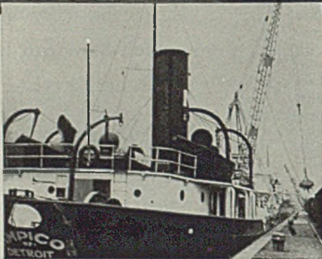
EC&M No. 6 Type SA 65-inch diameter Lifting Magnet on Freighter "Tampico," owned and operated by Nicholson Transit Co. of Detroit, which has paid for itself many times over through high speed loading and unloading during several seasons of successful operation.
