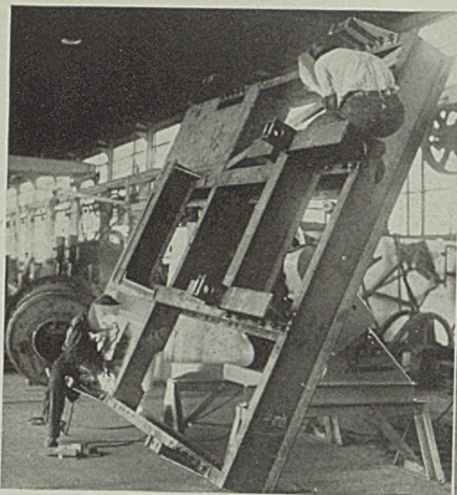
Left, positioner may handle large work by supporting unit from floor as shown here. Right, positioner is especially helpful in welding circular or cylindrical objects. Courtesy Ransome Concrete Machinery Co., Dunellen, N. J.
