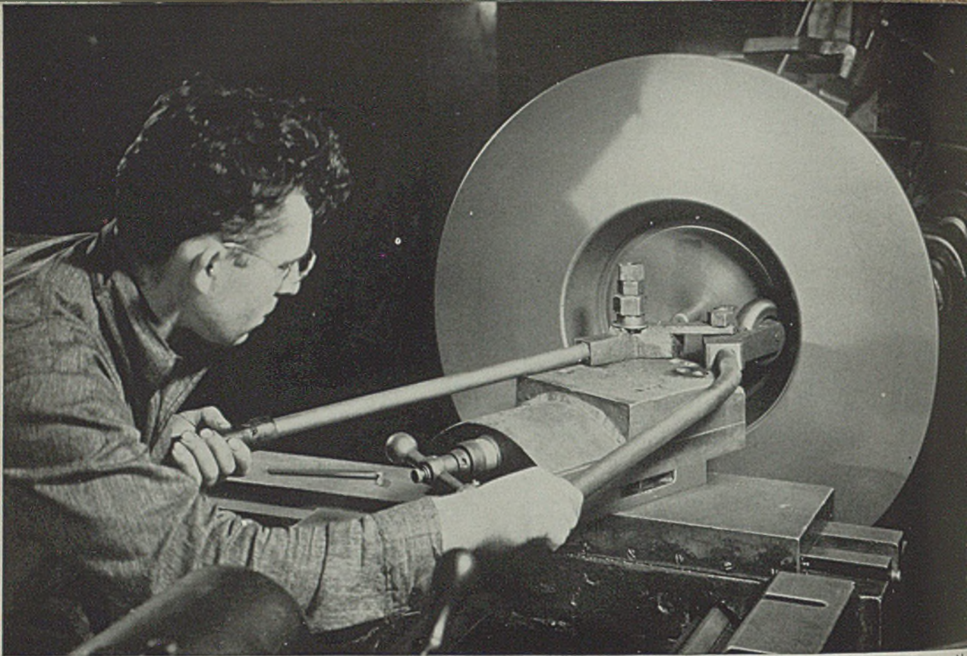
Fan scrolls for home-heating hot air fans are easily spun with Inland 16 ga. cold rolled deep drawn steel sheet. The fan scrolls are spun to a depth of 4-3/4 in. from Inland 16 ga. cold rolled deep drawn steel sheet.
