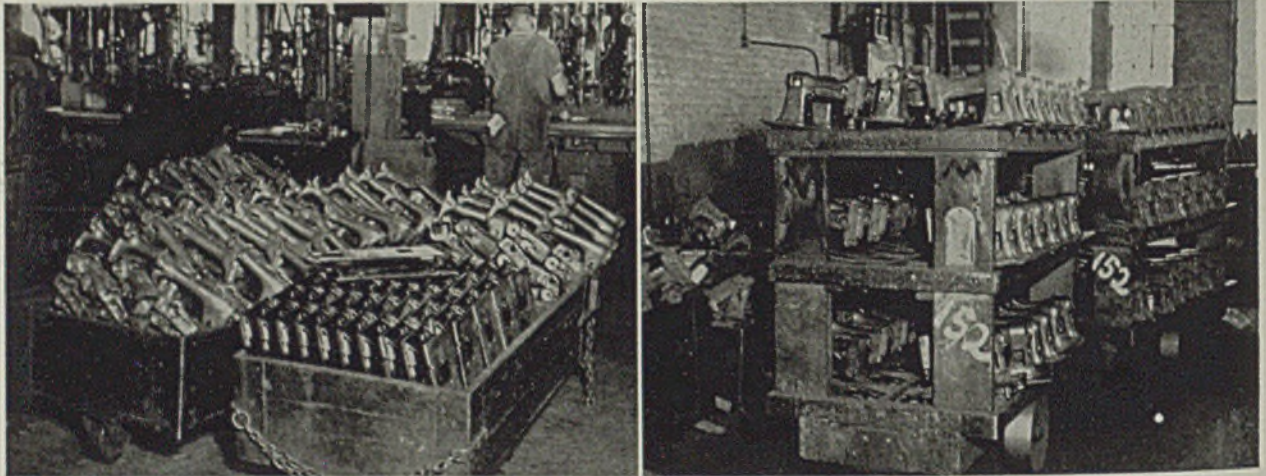
Fig. 1. (Left)—Arms and bed plates are transported to the machine shop in wood box trucks. Fig. 2. (Right)—After the bed plates and arms are assembled as one unit they are sent to the enameling department in 3-deck wood trucks
