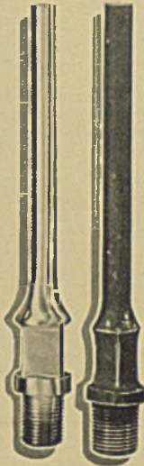
Duronze sucker rods before and after 18 1/4 months' service in an extremely corrosive well.
