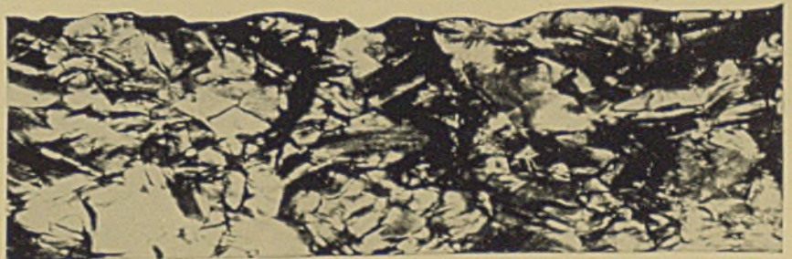
Figure 1. COARSE GRAIN. Longitudinal edge section of brass sheet after etching and then stretching. Mag. 15X.
