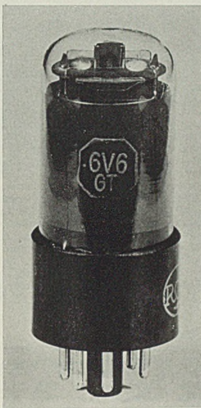
Fig. 1—Zirconium "getters" make possible high vacuum at low cost—an essential for modern radio receiver tubes
