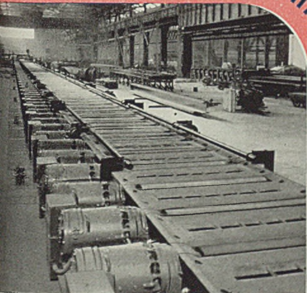
D-C DRIVE FOR RUNOUT TABLES. G-E direct-current motors in the 54-in. hot-strip mill. The steel industry continues to recognize the advantage of direct-current motors with Ward Leonard control for runout tables and coilers in wide-hot-strip mills. This is another G-E contribution to better, more economical steel-mill operation.
