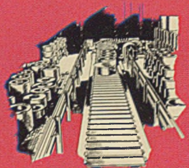
Pallet Conveyor for handling hot or cold coils.
