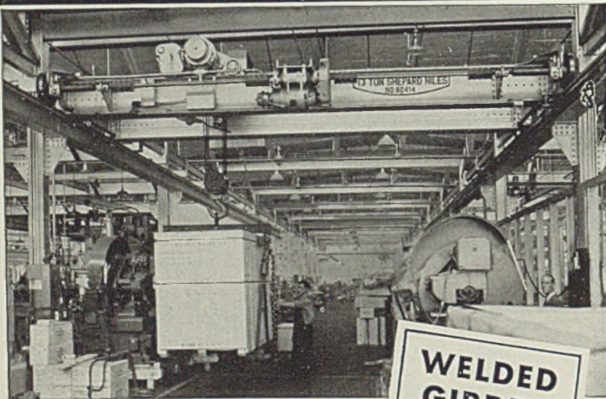
• Welded Box Girder Crane equipped with Shepard Niles 5-Speed Push Button Control for hoist, trolley and bridge motors.
