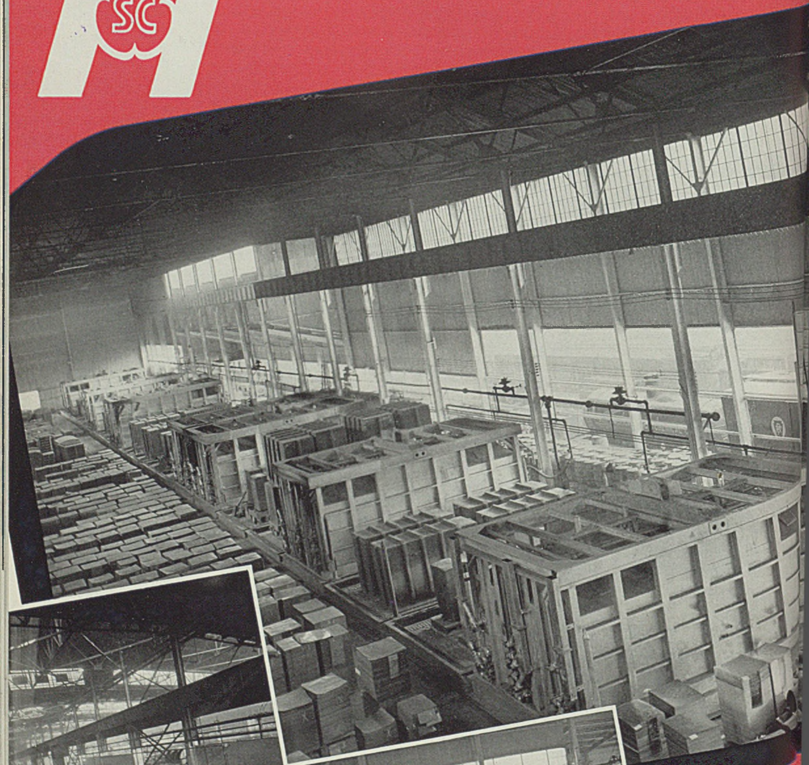
Above: Six of 12 SC covers at the Steubenville tin mill. Left: Double row cover at Steubenville tin mill. Center bank of radiant tubes permits the heating of a large tonnage under one cover.
