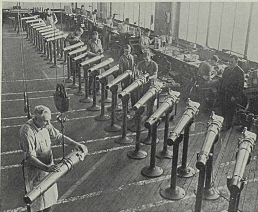
■ These 75-mm. howitzers, produced under scrutiny of Army inspectors at the Erie, Pa., works of General Electric Co., are rated as having the highest striking power for their weight of all the Army's guns. They will hurl 14-pound projectiles 9500 feet. Workmen in the plant's motor department are hand-finishing and fitting the howitzers. NEA photo
