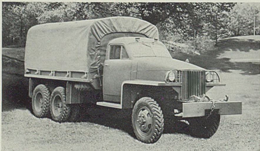
■ First of many thousand Studebaker army trucks ordered by the War Department recently was completed at the company's plant in South Bend, Ind. They are 6-wheel drive cargo vehicles of 2½-ton capacity
