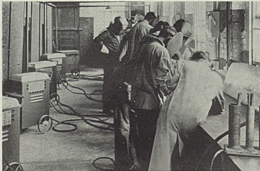
Any program for training welding operators involves a goodly amount of actual welding practice—anywhere from 80 to 200 hours. Here a group of students are using five 200-ampere Westinghouse transformer-type welding sets to "get the feel" of alternating-current welding
