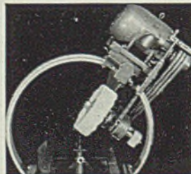
Ring-type, floating polishing head—exclusive on Udylite full automatics. Easily adjusted. Provides right pressure at all points.
