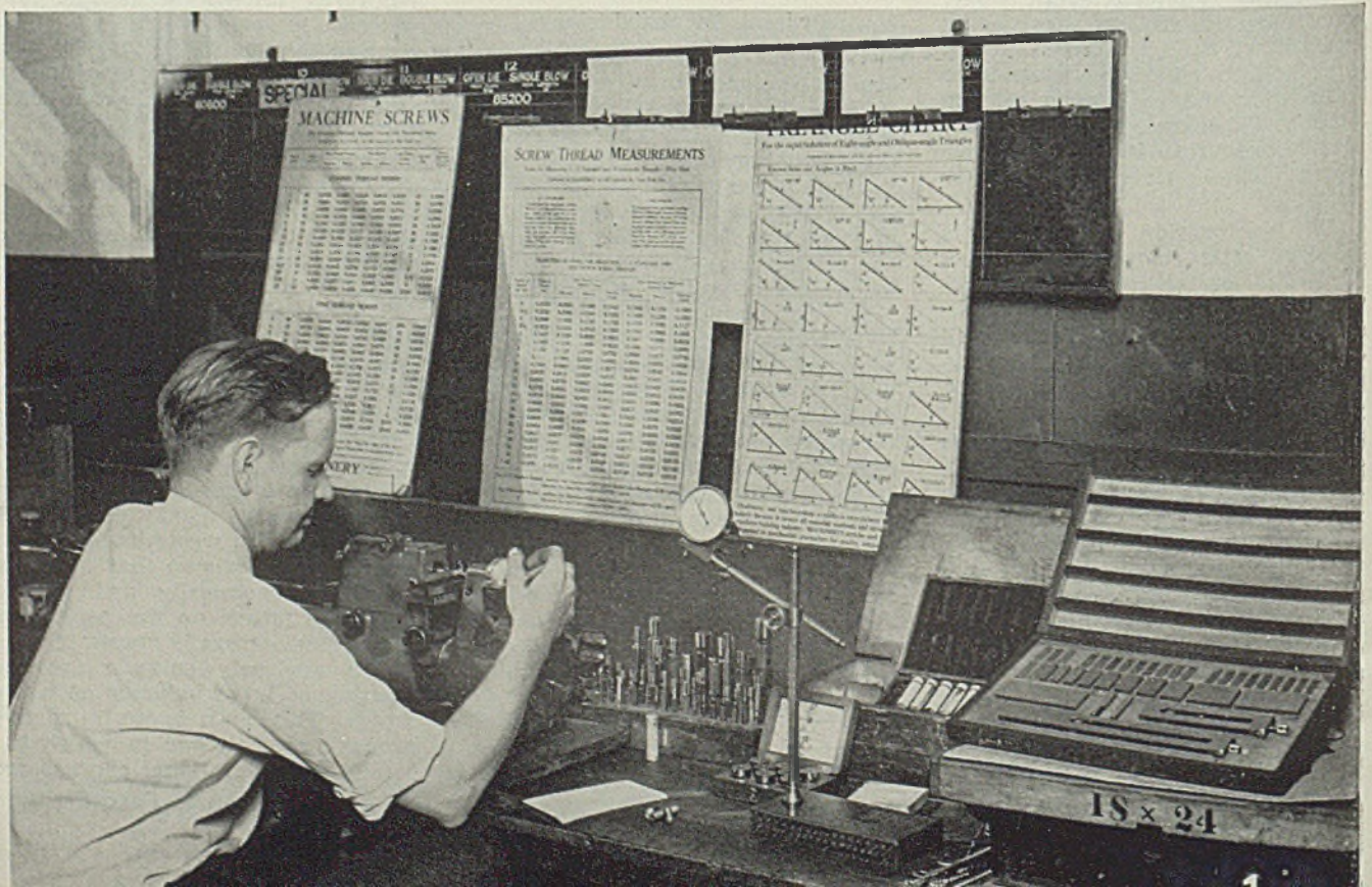
Fig. 1—Part of the master tool section. Note special plug gages, Jo blocks, and other equipment. The operator is using a supermicrometer
