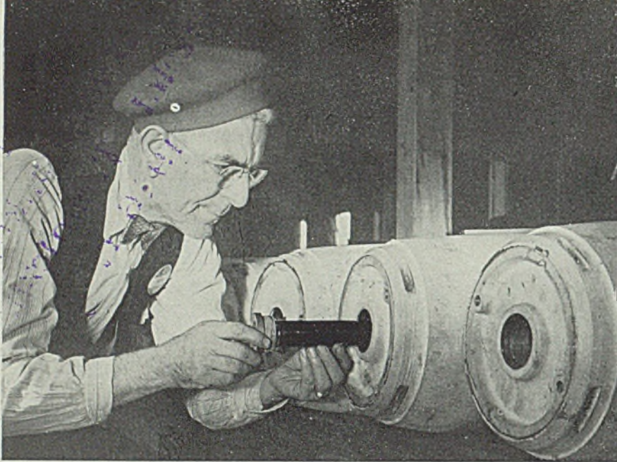
■ The 500-pound bomb is completed by inserting a steel explosive container in the nose. This part supplies one of two explosions which occur when the missile hits its mark
