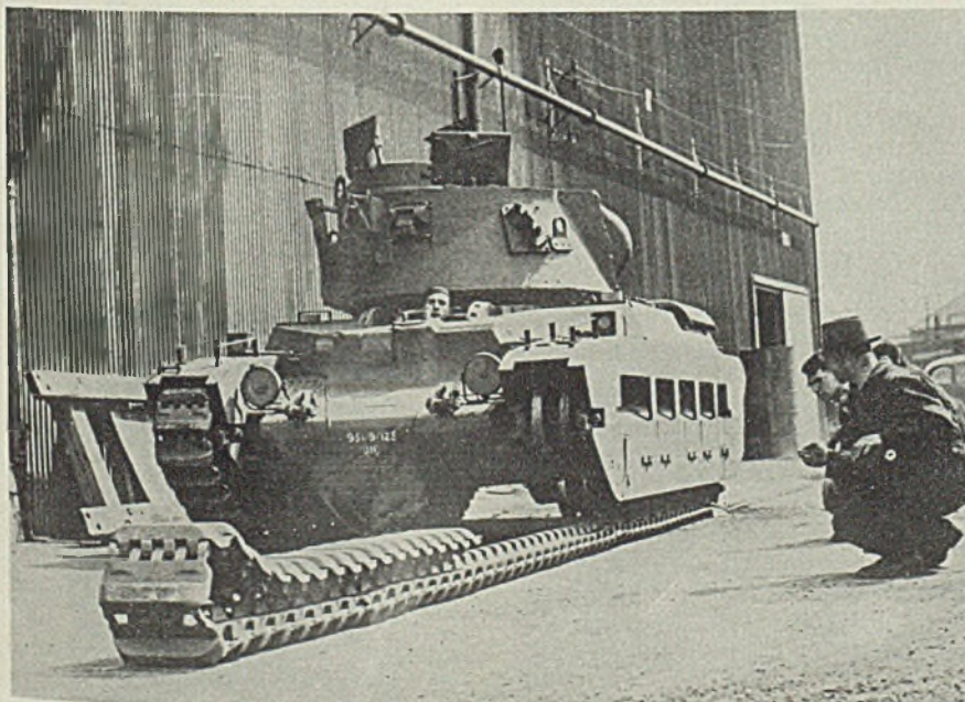
■ Mounting the track is the last step in production of this heavy tank, manufactured in England. The tread is extended and the tank driven onto it, after which the ends are fastened together to form an endless track. NEA photo passed by the British censor
