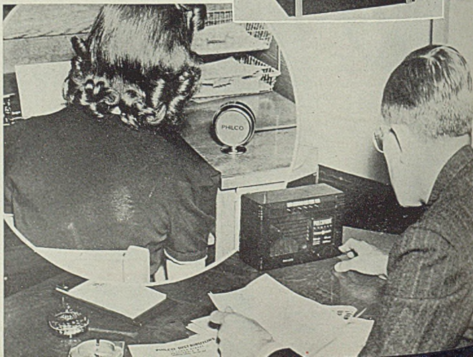
Fig. 4—A talk-back unit like this Philco allows a person at other end to communicate back to the master station. Any number of outlying stations can be hooked up in such a system, or all can be selector-transmitters allowing a person to call and talk with any station from any other station in the system or all of them simultaneously
