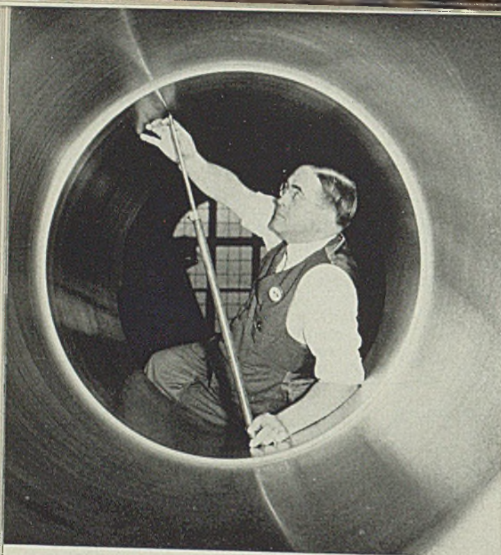
Fig. 9—Measuring inside of a hoop for a large gun at Wattervliet. O.E.M. photo by Palmer
