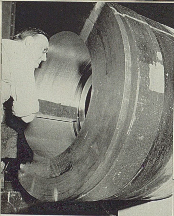
Fig. 6—Machining operations, above, at Watervliet Arsenal on the seat for the breech block of a large-sized rifle: O.E.M. photo by Palmer
