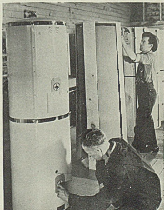
Fig. 7—Here completed electric hot water tanks are being inspected and crated for shipment. Note the 8-sided crates employed and the steel strapping around the center of the crate sections
