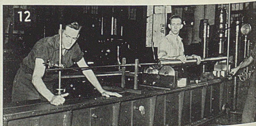
Fig. 11—This shows how a transverse saw cut is made on the breech end of the gun forging in order to obtain a transverse test specimen
