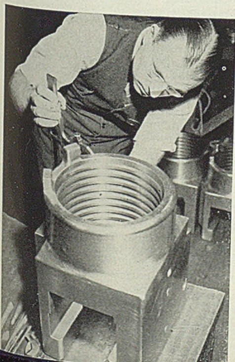
Fig. 7—Inspecting a breech ring. O.E.M. photo by Palmer
