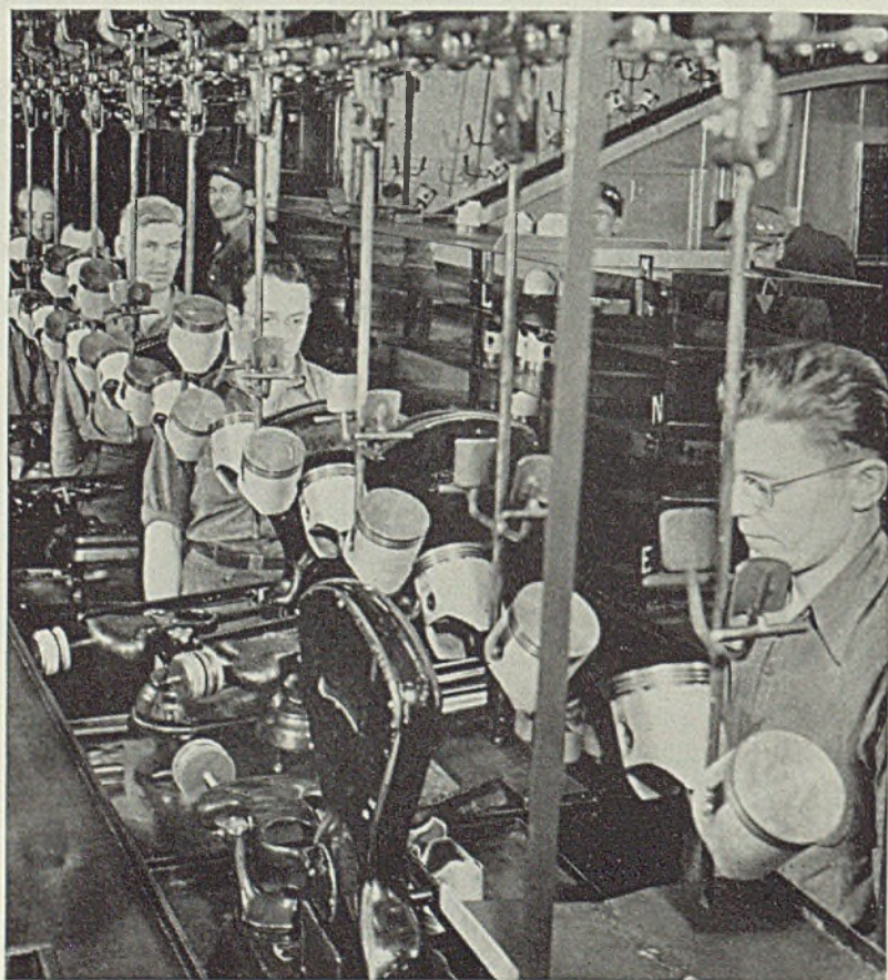
■ Endless stream of pistons on conveyor at Chevrolet plant in Flint, Mich., passes line of operators who weigh and check balance of each piston on specially designed scales. No part of the modern engine is more carefully designed, machined and inspected than the piston, which takes the direct impact of the cylinder explosion. In more than 20 years of manufacturing experience Chevrolet has produced 85,000,000 cast iron pistons
