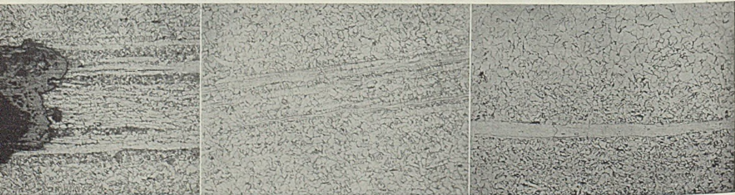
Fig. 8—Views of defect, left to right. A contains some foreign material; B is a continuation of the ghost in A. C shows almost the end of ghost
